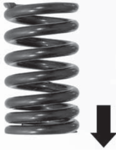
Figure 12-31 The valve spring should be installed with the compressed coils facing the nonmoving part of the engine. Copyright by American Honda Motor Co., Inc. and reprinted with permission.
