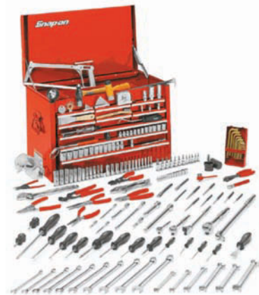
Figure 3-1 A typical set of hand tools that a power equipment engine technician would own. This assortment of tools could be used for different applications and isn't limited to power equipment engine repair. Courtesy of Snap-on Tools Company.
