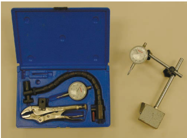
Figure 3-52 Two dial indicators. The one on the right uses a magnetic base to hold it in place, whereas the one on the left uses a flexible shaft that locks in place.
