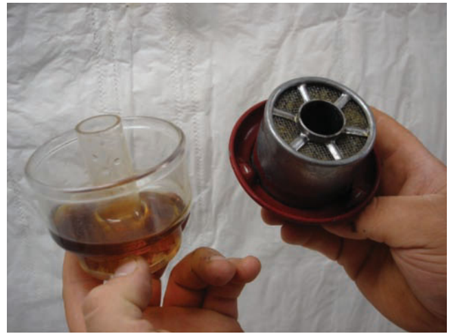
Figure 16-40 An oil bath air filter directs incoming engine air over an oil sump that catches dirt particles. This filter can be seen in older engines.
