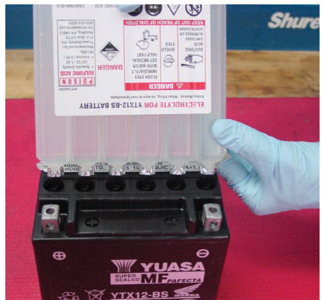
Figure 14-21 The acid pack is installed using the manufacturer's instructions.
