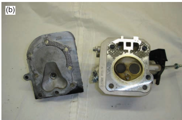
Figure 12-12 A comparison of (a) the tops and (b) the underneath of the L-type and OHV engine heads.
