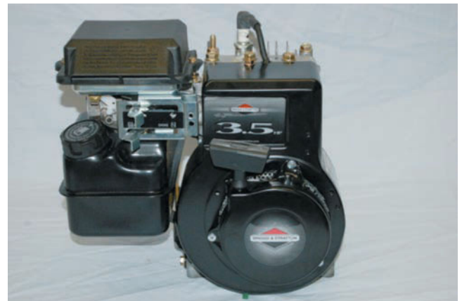
Figure 5-30 The most common type of power equipment engine is of the single cylinder variety.
