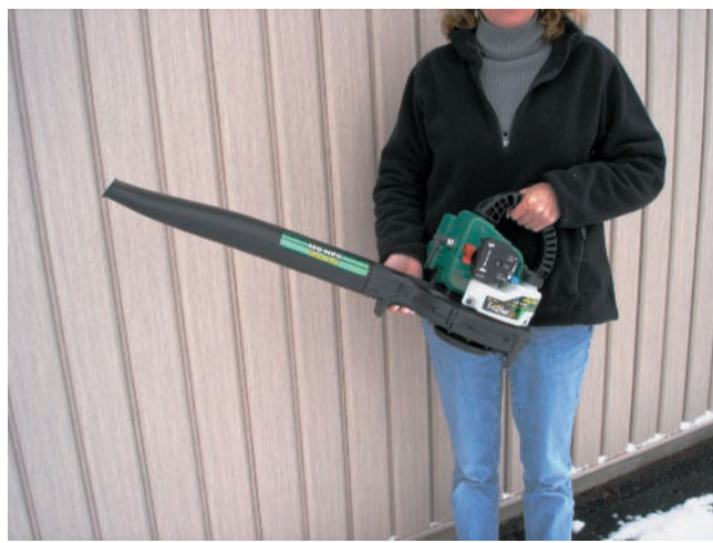
Figure 10-1 Two-stroke engines in today's power equipment are found primarily on small handheld units such as gas-powered blowers.
