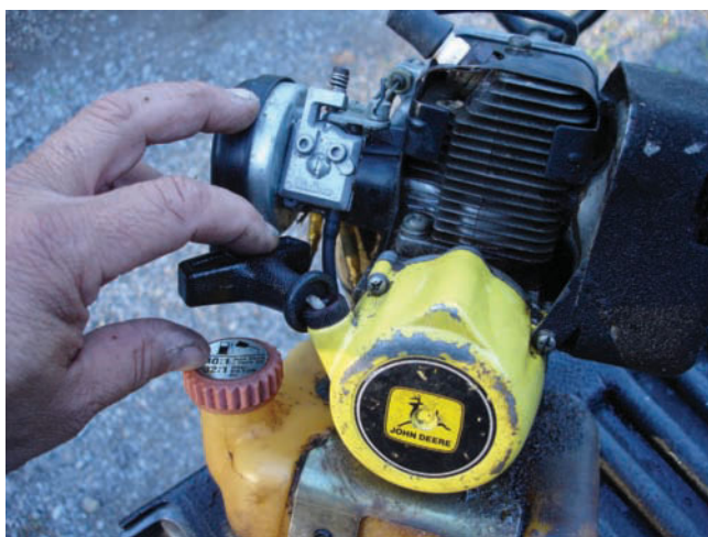
Figure 8-38 A diaphragm carburetor can be turned in any angle without impairing operation.
