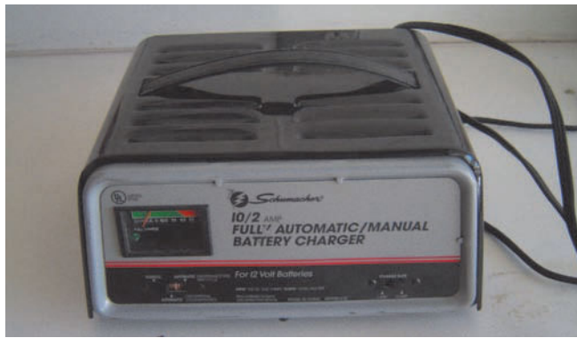
Figure 14-44 Automotive-type constant voltage battery chargers are not usually recommended to charge smaller power equipment batteries.
