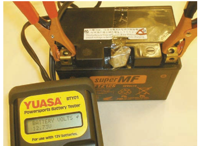
Figure 16-28 Battery conductance analyzers are becoming more popular in the motorcycle industry due to their ability to more accurately tell us the condition of the battery.
