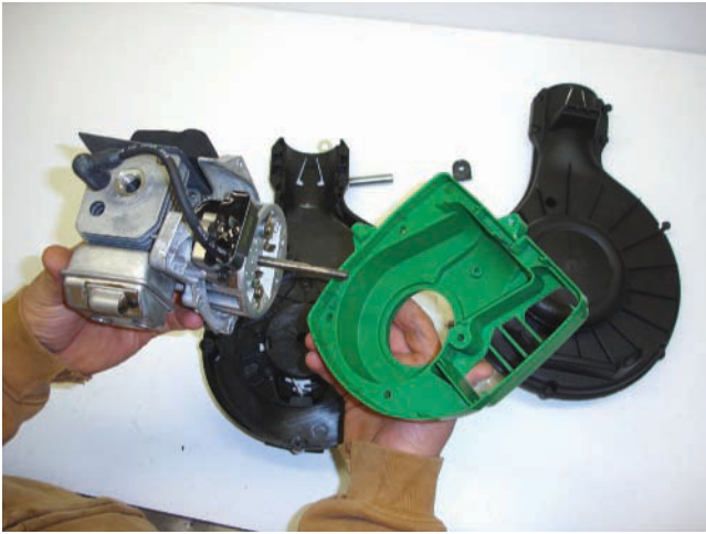
Figure 11-3 To gain access to the two-stroke engine bottom end components, you must first remove the engine from the implement it's powering.
