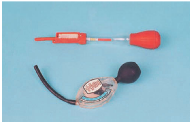
Figure 16-9 A hydrometer is used to check if the mixture of coolant and water is correct.
