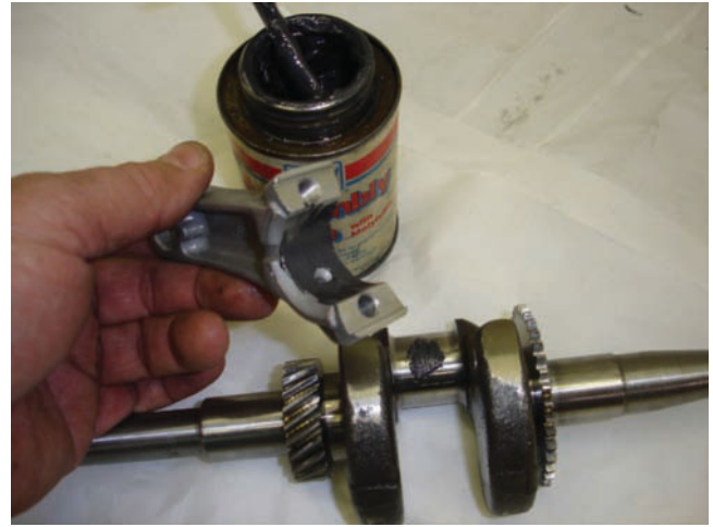
Figure 12-90 Using an assembly lubricant on the bearing surfaces is important to assist with additional lubrication during initial start-up of the engine.
