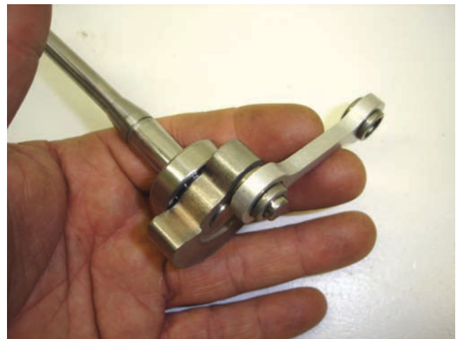
Figure 11-15 Crankshafts in small two-stroke power equipment engines are often single-piece units that look like one half is missing.
