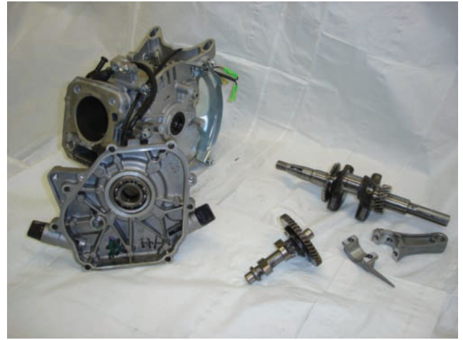
Figure 12-72 The primary components of the bottom end of a typical power equipment four-stroke engine.
