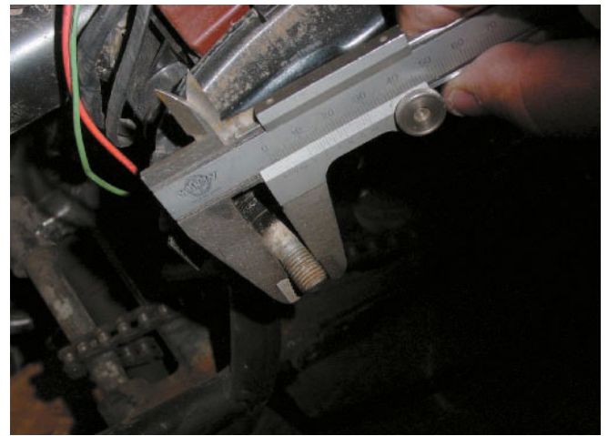
Figure 3-47 A vernier scale caliper is shown being used here.
