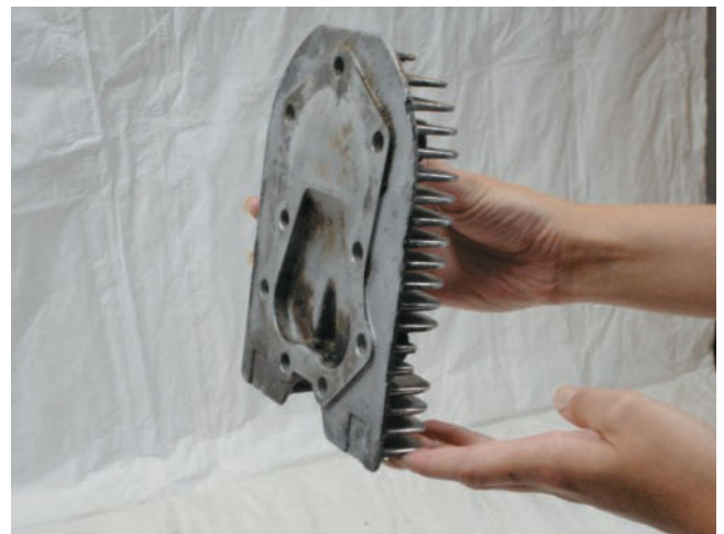
Figure 5-19 Heads on engines that have the valve mechanism in the cylinder block have no moving parts. Note the fins that are used to assist in cooling the engine.
