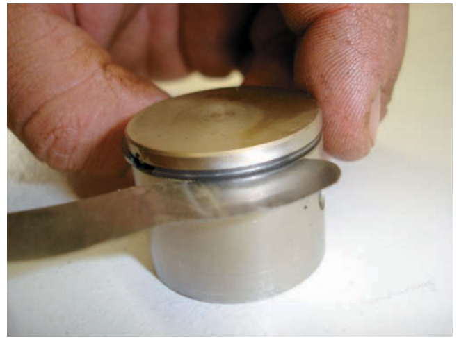
Figure 10-20 Measuring ring side clearance.
