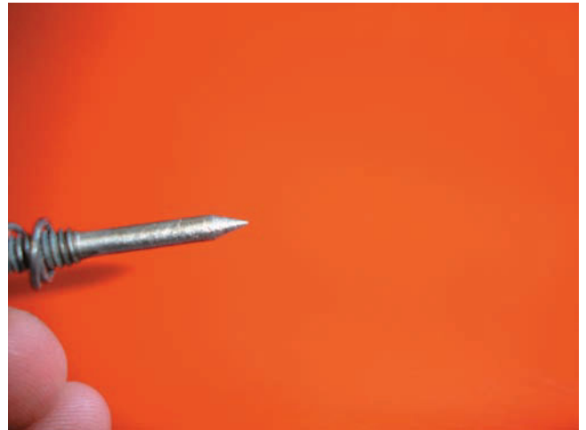
Figure 8-12 The tip of the low-speed mixture screw is pointed, to allow for a more precise adjustment.
