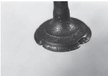
Figure 12-26 A common cause of burned valves is excessive heat.
