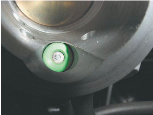
Figure 8-51 Various types of tips can be found on a fuel injector. Decisions on the type of injector to be used can be based on intended use as well as cost.
