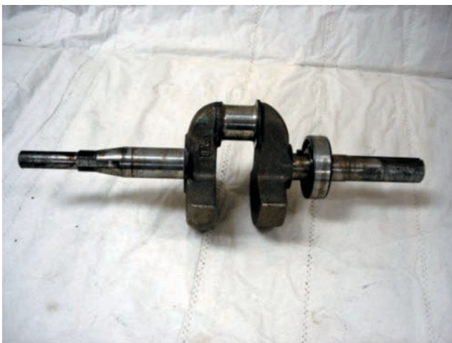
Figure 6-16 A one-piece crankshaft used in four-stroke engines.
