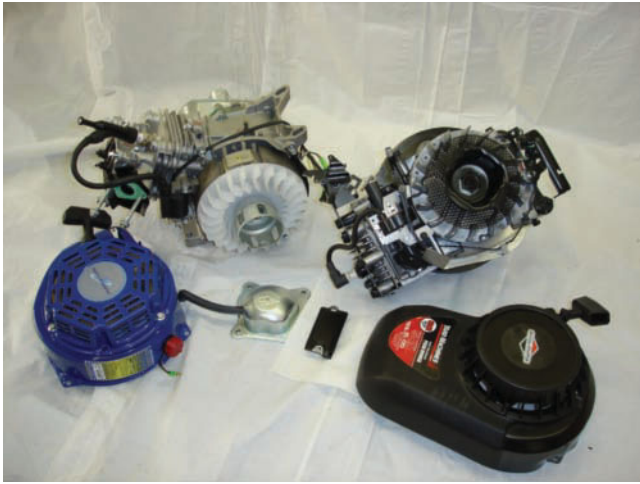
Figure 12-8 After the covers have been removed, it's easy to get at the engine's internal components.
