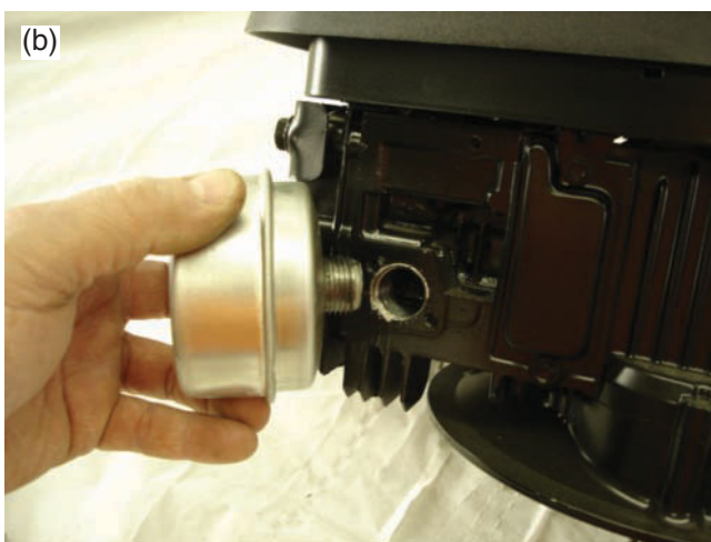
Figure 12-6 Removing the mufflers on the engine helps gain access to covers that will need to be removed. Note that the OHV engine (a) has a bolt on the muffler, whereas our L-head engine (b) has a muffler that screws on.
