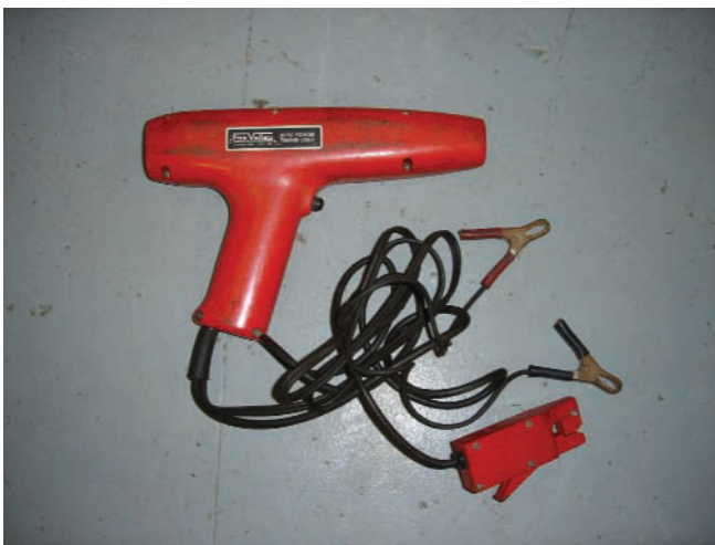
Figure 16-30 A tool that isn't often used any longer due to the advent of electronic ignition systems; the timing light can be used to verify the correct ignition timing of an engine, by pointing its flashing light at the flywheel while the engine is running.
