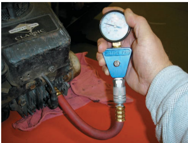
Figure 16-12 A typical compression gauge attached to a cylinder.
