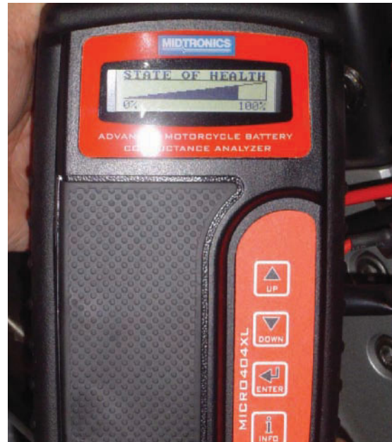
Figure 14-48 A battery conductive analyzer has the capability to test the state of health of a battery.
