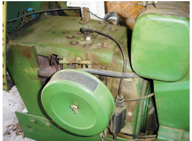
Figure 5-28 This air-cooled engine is completely covered in shrouds. Air-cooled power equipment engines use an engine-driven fan attached to the flywheel to move air and keep the engine running cool.
