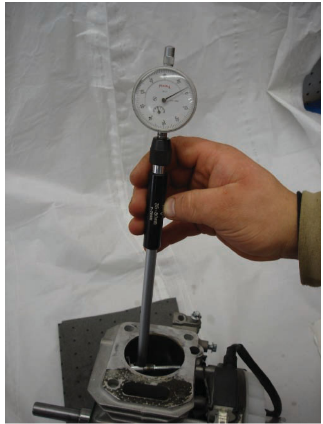
Figure 12-67 Using a cylinder bore gauge to measure the inside diameter of the cylinder.
