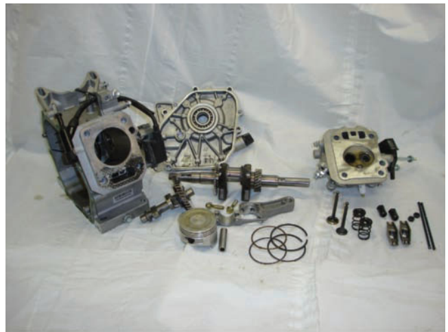
Figure 12-4 The components found in a typical OHV power equipment engine.
