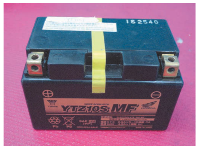
Figure 14-22 Some MF batteries come prefilled with acid from the battery manufacturer.
