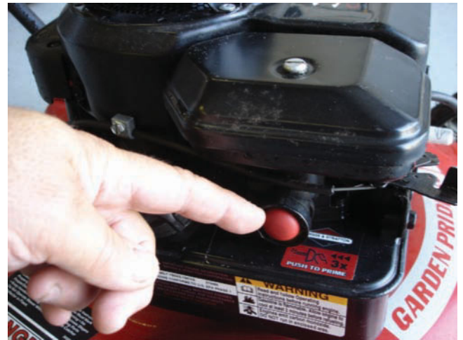
Figure 8-18 A primer cold start system pushes fuel directly into the engine.
