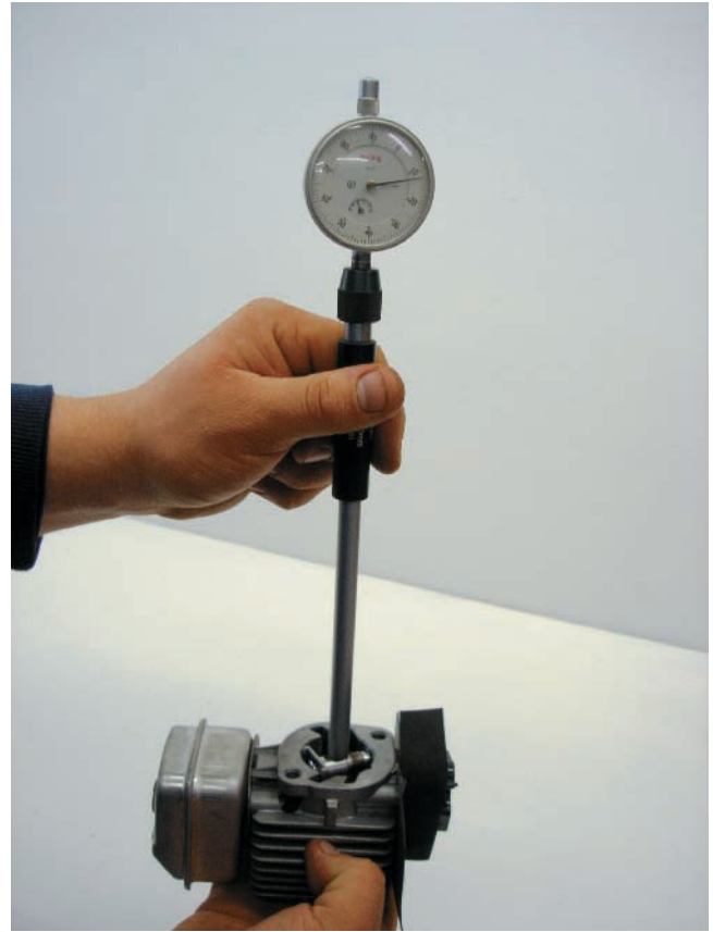
Figure 10-8 The measuring of the bore of the cylinder with a dial bore gauge.
