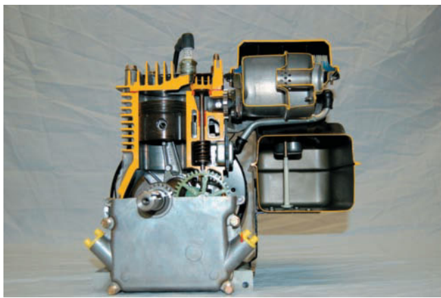
Figure 6-18 A cutaway of a one-piece engine crankcase (also known as a block). All the components of the engine are contained in or on the block.
