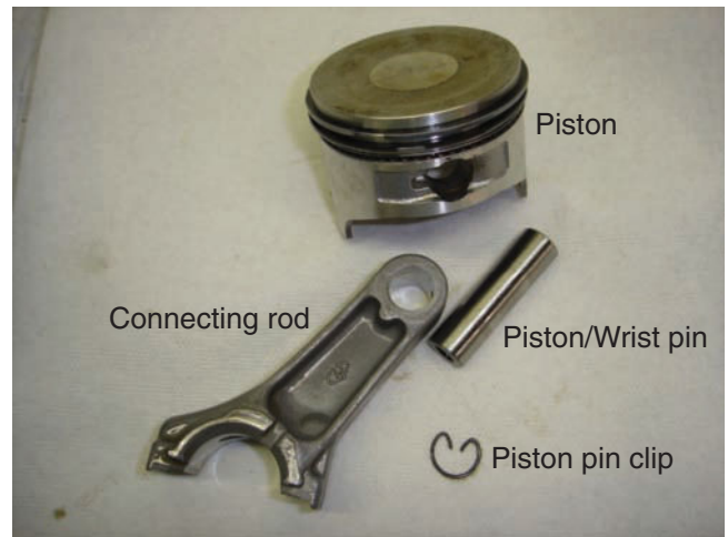
Figure 12-51 The piston pin connects the piston to the connecting rod and is held in place by piston pin clips.
