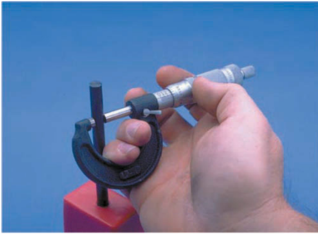
Figure 3-51 Measurement using a micrometer.
