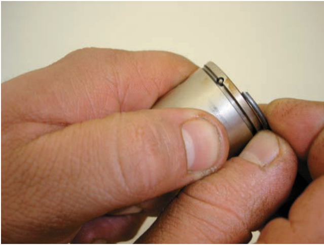
Figure 10-17 When removing the piston ring, be careful not to spread the ring too much or else damage may occur.
