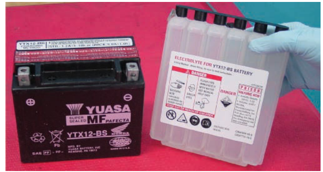
Figure 14-20 Most MF batteries come with their own acid pack, which must be installed prior to initial use.
