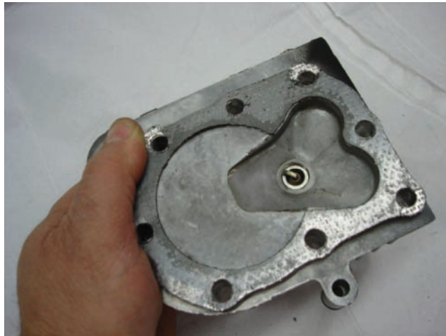
Figure 12-9 The L-head engine has no moving parts attached to it. Shown is the underside of the head.
