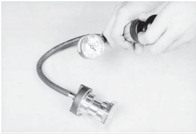
Figure 7-27 A cooling system tester can be used to perform a radiator cap pressure test.
