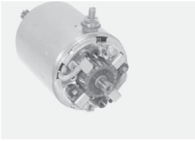
Figure 15-33 The end cap of this starter motor has been removed to show its brushes, brush springs, and commutator. Copyright by American Honda Motor Co., Inc. and reprinted with permission.
