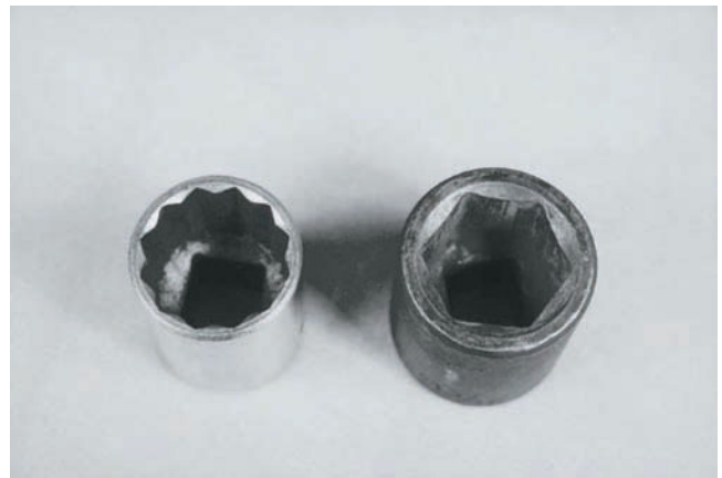
Figure 3-14 Six- and 12-point sockets. Whenever possible, it's recommended that a 6-point socket be used as it's stronger.
