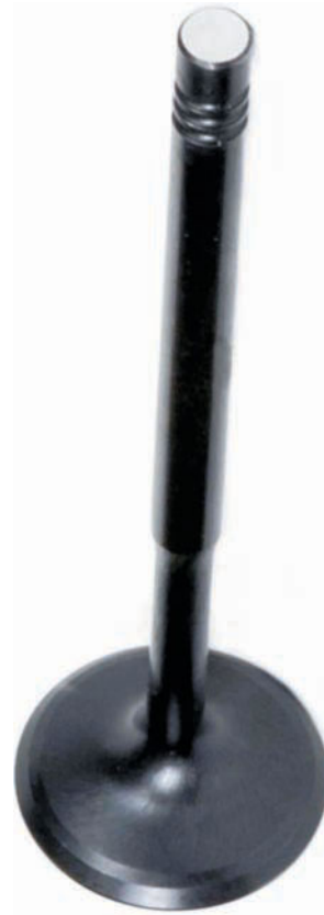
Figure 5-21 The valves in a four-stroke engine control the air–fuel mixture that’s drawn into the cylinder and the exhaust gases that are expelled.
