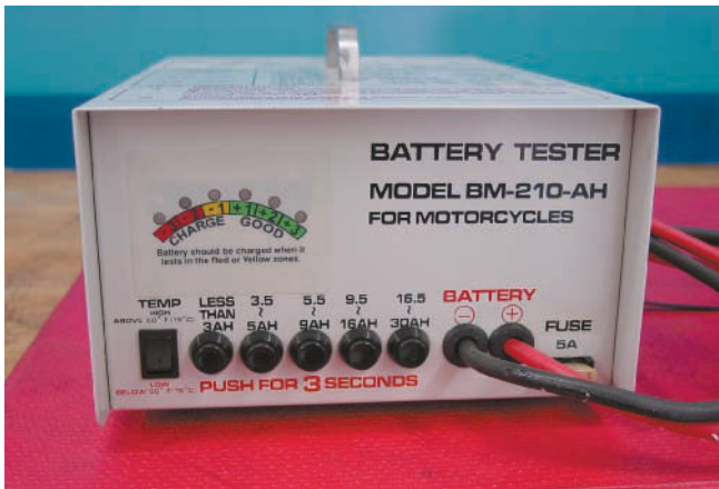
Figure 16-27 A battery load tester places a load on a battery to check its ability to withstand current flow through it.
