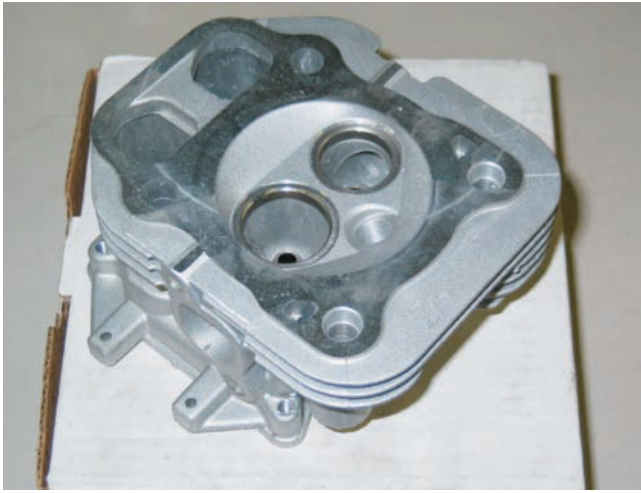
Figure 5-20 Engines that contain the valve mechanism in the head are more complex and contain holes that are called ports. These ports are opened and closed with valves.
