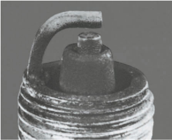
Figure 16-18 A fuel-fouled spark plug has dry, black, fluffy carbon deposits on the plug electrodes. Courtesy of Federal-Mogul Corporation.
