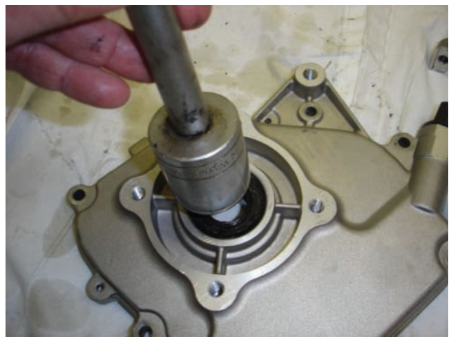
Figure 12-78 When installing seals, use a tool that will not damage the seal, as shown here.
