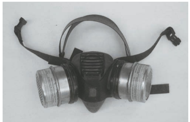
Figure 2-13 Whenever there is a danger of breathing harmful fumes, use a high-quality respiratory breathing protector.
