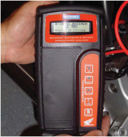
Figure 14-47 A battery conductive analyzer describes the battery's ability to conduct current. This type of test is a more accurate way to determine the battery's internal condition compared to load testing.
