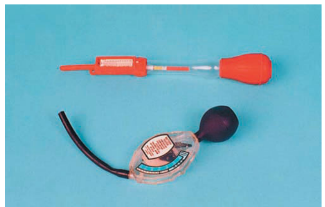
Figure 7-32 Two hydrometers are shown here. Hydrometers are used to measure the specific gravity of a liquid. When antifreeze is added to water, the hydrometer measures the weight change.
