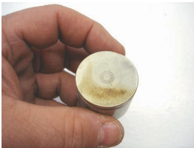
Figure 10-14 An examination of the piston crown is mandatory to ensure no damage has occurred.
