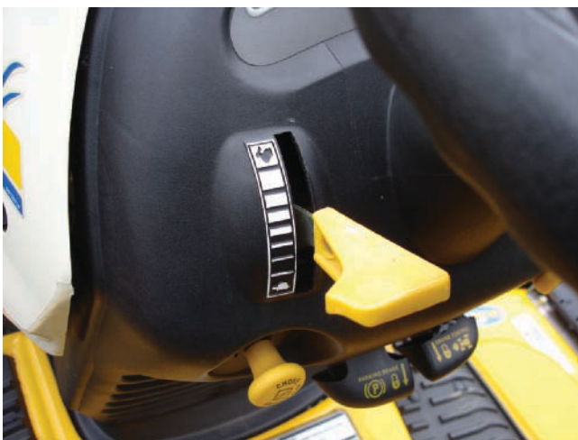
Figure 9-1 Engines with manual throttle control often use a control linkage as the throttle may be operated at a distance from the carburetor. Shown is a throttle control mechanism on the dashboard for easy access.
