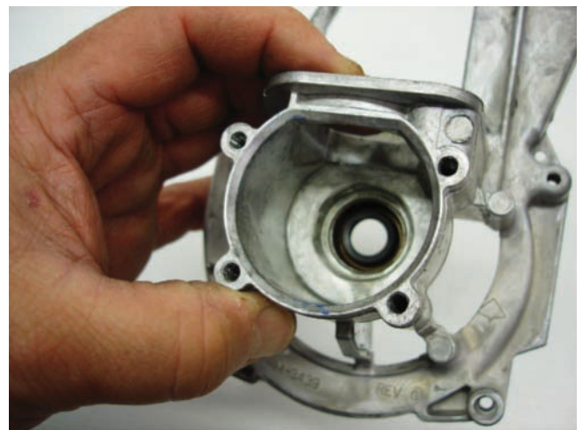
Figure 11-5 When inspecting the crankcase, look closely for cracks, loose-fitting bearings, and worn out fastener anchoring points.
