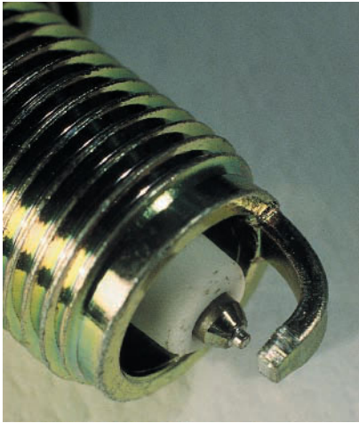
Figure 15-10 A platinum-tipped spark plug. Courtesy of Bob Freudenberger.
