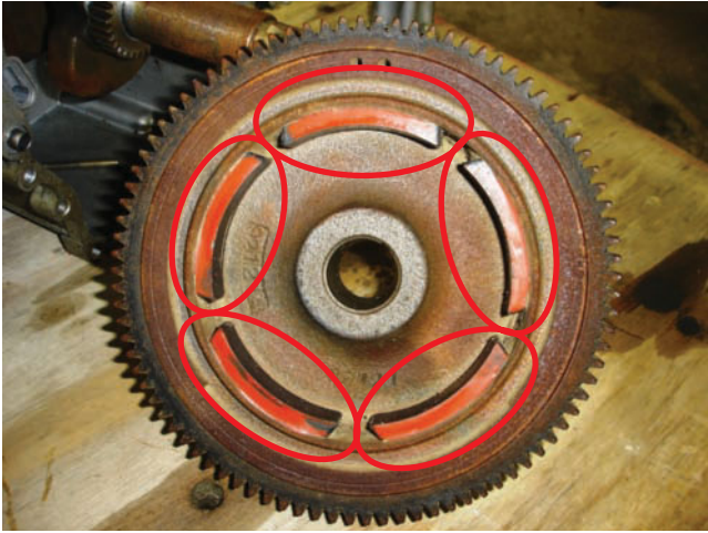
Figure 14-5 Permanent magnets are attached to the rotor.
