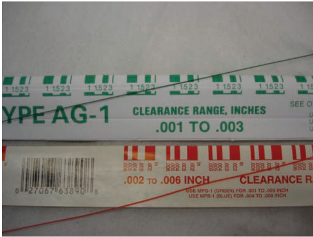
Figure 12-82 Plastigage comes in various colors that relate to different sizes.
