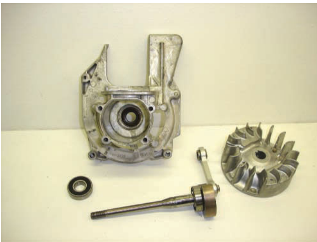
Figure 11-4 In most cases in two-stroke power equipment engines, disassembly is quite simple, as there are not many components, as seen here.
