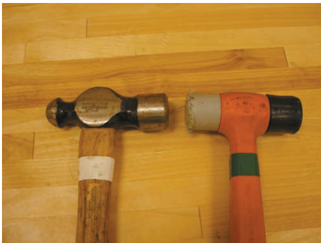
Figure 3-29 The ball peen hammer (left) and rubber mallet (right) are among the most commonly found in a power equipment engine technician's toolbox.
