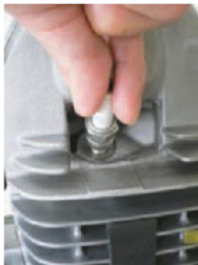
Figure 16-22 To reinstall a spark plug, don't force it into the hole; hold the plug with your fingers or with the correct spark plug socket, and gently screw the plug into the threaded cylinder head opening.
