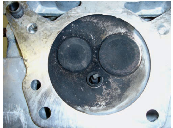
Figure 12-14 Carbon buildup is a hard residue that's found often on surfaces exposed to the burned air-fuel mixture, as seen in this combustion chamber.
