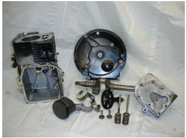
Figure 12-3 The components found in a typical L-head power equipment engine.
