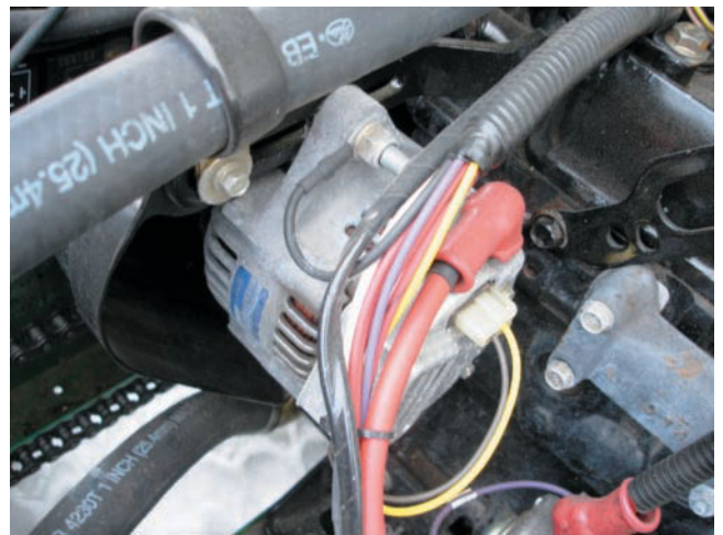
Figure 14-33 An excited-field charging system isn't generally located on the crankshaft, as seen here.
