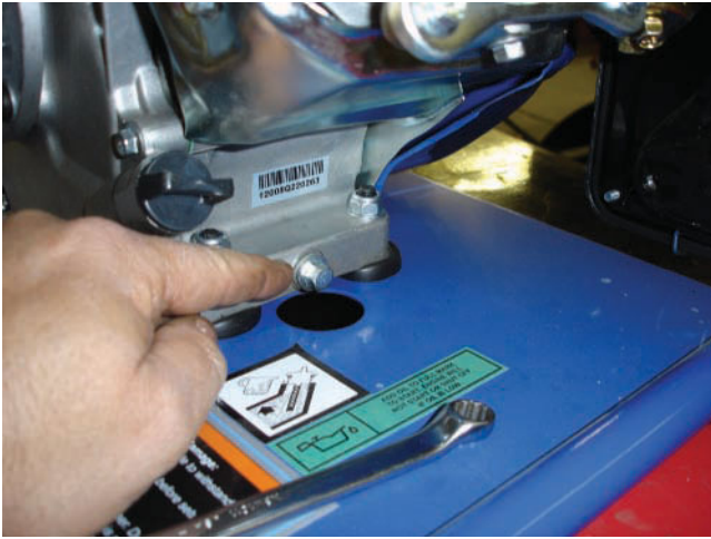
Figure 12-5 The oil drain bolt in an OHV power equipment engine.
