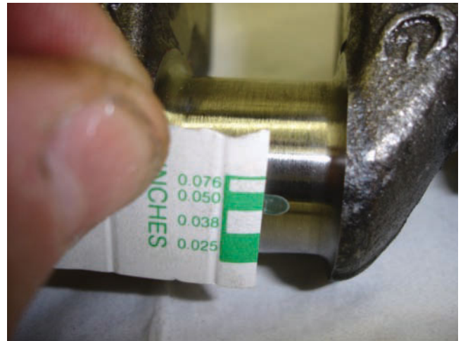
Figure 12-84 Measuring the clearance of the bearing surface.
