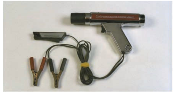
Figure 3-58 Timing lights are still popular and are used to determine if the engine's spark timing is correct.
