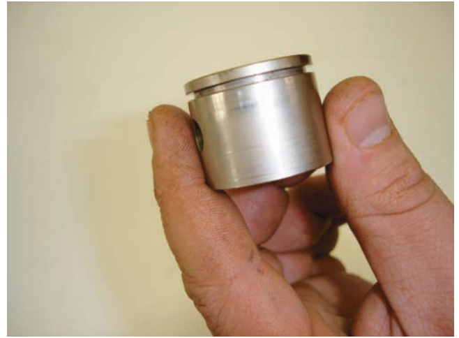
Figure 10-12 A visual inspection of the piston includes checking for cracks or any other signs of surface damage, such as scratches or score marks.
