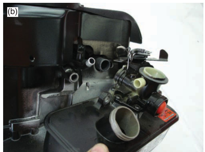
Figure 12-7 Carburetor removal in an OHV engine (a) and an L-head engine (b).
