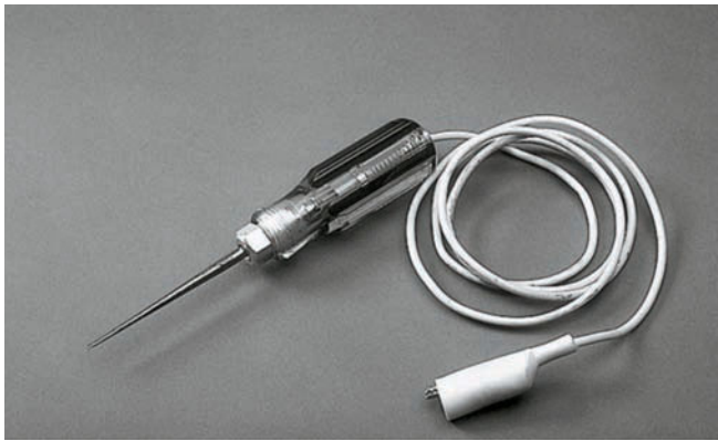
Figure 3-59 A test light is a handy tool when diagnosing a problem in an electrical system. There are two types of test lights, self-powered and non-self-powered. Shown here is a non-self-powered test light.
