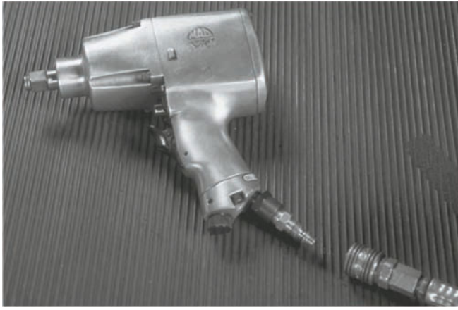
Figure 3-43 A typical air-power impact wrench. These types of tools should be used only to remove items and not used to install, as they're so powerful that they could break or over-torque the fastener in question.
