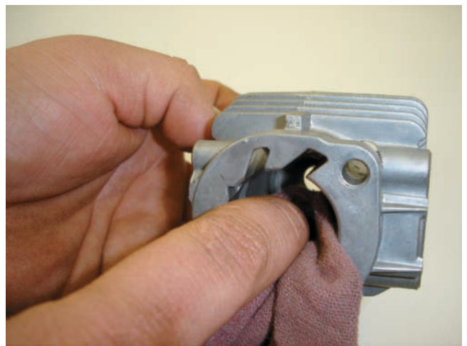
Figure 10-23 It's important that cylinders be cleaned thoroughly before assembly.
