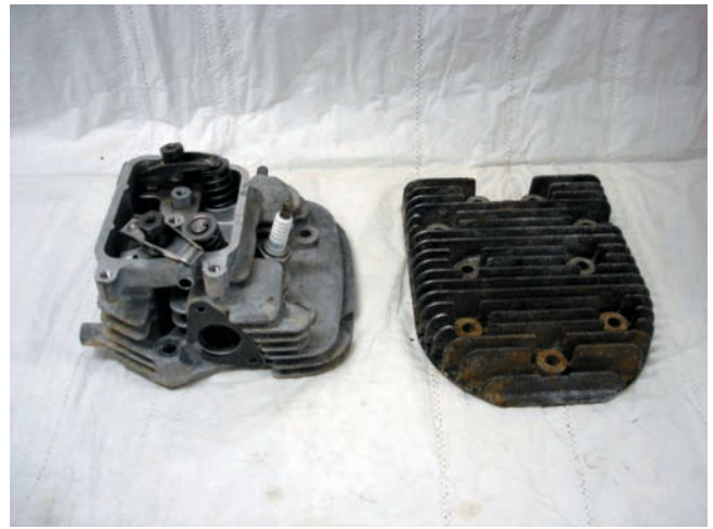
Figure 6-3 There are two basic types of cylinder heads in power equipment engines. The cylinder head on the left contains the intake and exhaust valve train components. The cylinder head on the right is more or less a cover for the cylinder, which caps the top of the engine.
