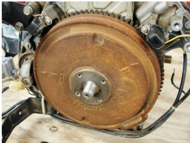
Figure 14-30 The alternator for the three-phase permanent-magnet charging system has the rotor mounted on the crankshaft. The stator is mounted on the crankcase.
