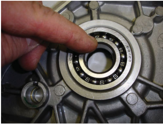
Figure 12-79 A technician inspecting the ball bearing race by hand while it's mounted on the crankcase.
