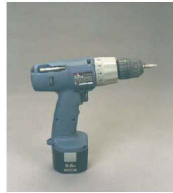
Figure 3-40 Self-powered drill motors are popular and can also be used as a powered screw driver, as seen here.
