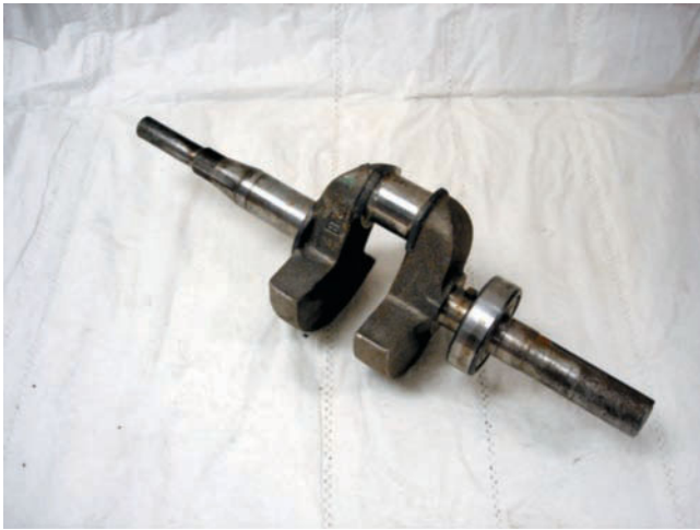
Figure 5-13 A one-piece crankshaft without the connecting rod.
