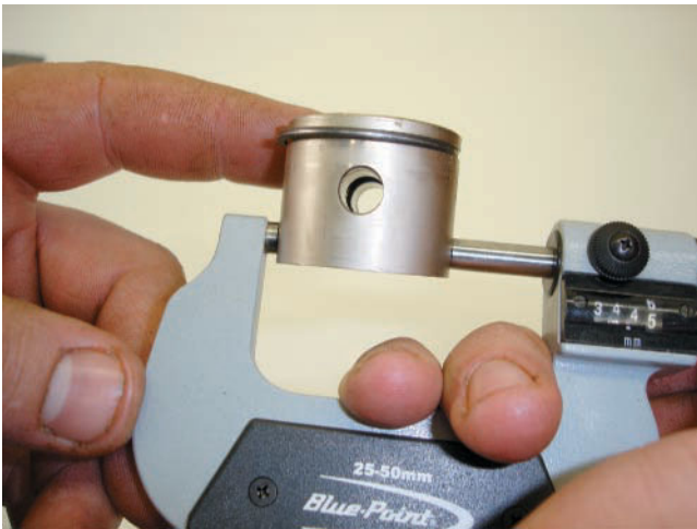
Figure 10-18 Measuring the piston with a micrometer.
