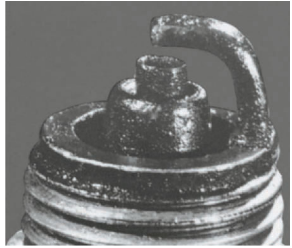
Figure 16-17 Oil fouling causes the plug to be saturated with shiny oil deposits. Courtesy of Federal-Mogul Corporation.
