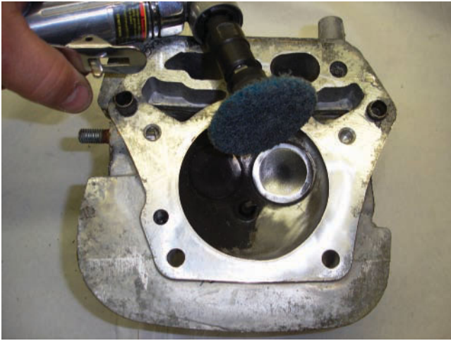
Figure 12-15 The combustion chamber after it's been cleaned of the carbon residue.
