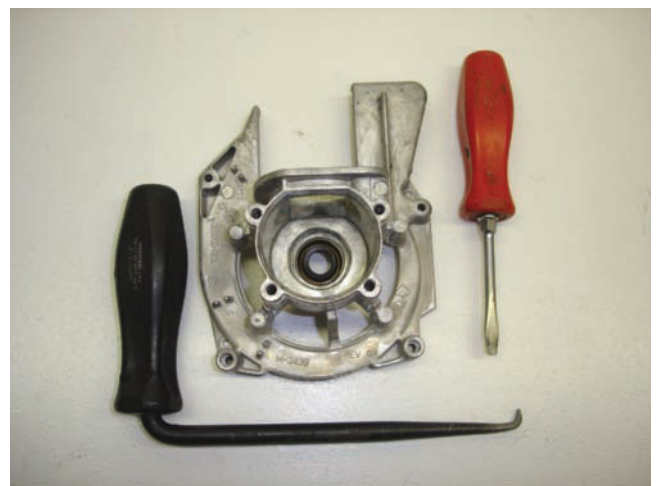
Figure 11-9 You can purchase special tools to remove seals or, in many cases, just pry it out with a screwdriver. Never reuse a seal once it has been removed.
