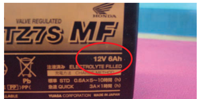
Figure 14-42 In some batteries, the amp-hour rating may be easily determined by looking at the battery cover. Copyright by American Honda Motor Co., Inc. and reprinted with permission.
