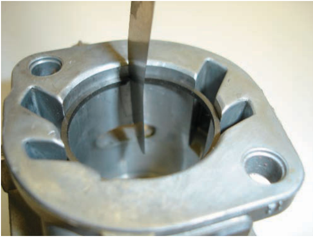
Figure 10-24 Measuring piston ring end gap with a feeler gauge.
