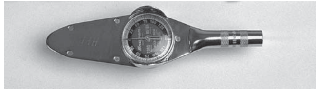
Figure 4-36 Dial-type torque wrenches are not used often on power equipment engines.
