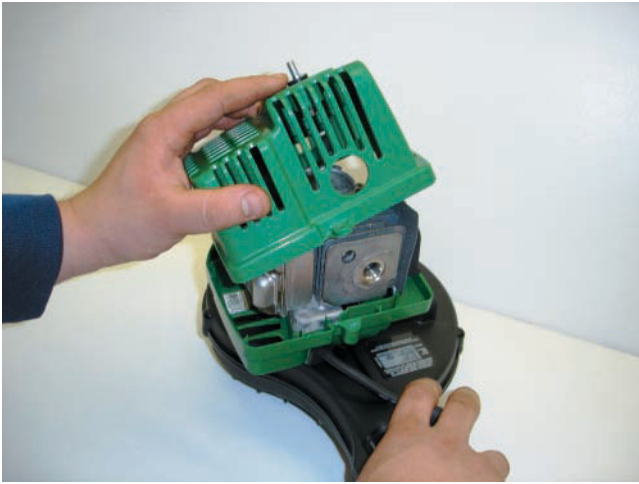
Figure 10-4 Removing the engine cover exposes the external components to the two-stroke engine's top end.
