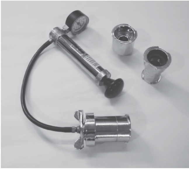
Figure 16-8 A typical cooling system pressure tester. This tool checks for leaks in hoses, pipe connections, radiator, and water pump.
