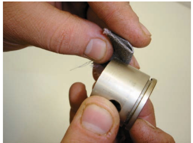
Figure 10-13 Minor scuffing can be removed by using a fine emery cloth to clean the surface of the piston.
