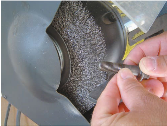
Figure 4-27 Cleaning a bolt using a wire wheel. Use proper safety apparel when using a wire wheel. Can you tell what safety apparel is missing in this picture?
