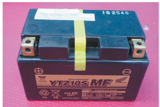
Figure 16-26 A maintenance-free battery has no filler caps, and some, like the one shown here, come from the factory pre-filled with acid.
