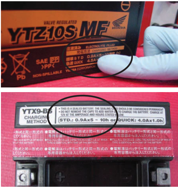
Figure 14-43 Some battery amp-hour ratings must be determined by locating the STD number. Multiply the STD number by 10 to determine the amp-hour rating. The STD rating may be shown on the front (top) of the battery or on the top of the battery (bottom).
