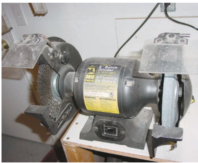
Figure 3-41 A typical bench grinder has a grinding wheel as well as a wire brush attachment.
