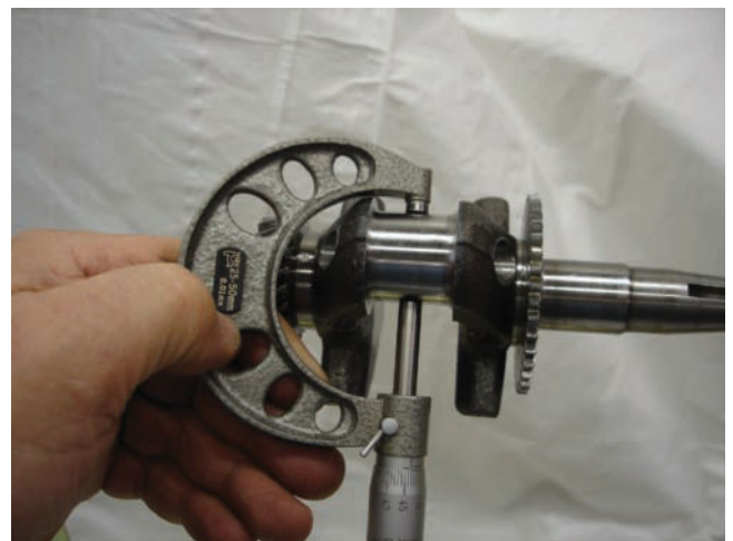
Figure 12-88 Measuring crankshaft-bearing surfaces with a micrometer.
