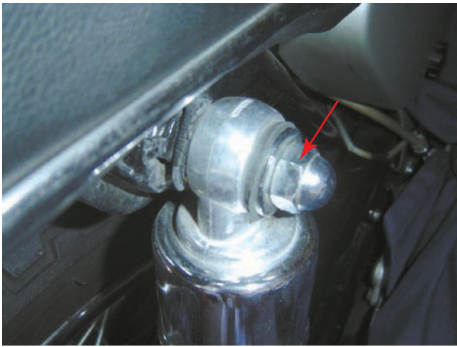
Figure 4-20 Acorn or cap nuts are used to cover threaded ends of bolts or studs. Install them correctly or else the nut will bottom out and not tighten properly.
