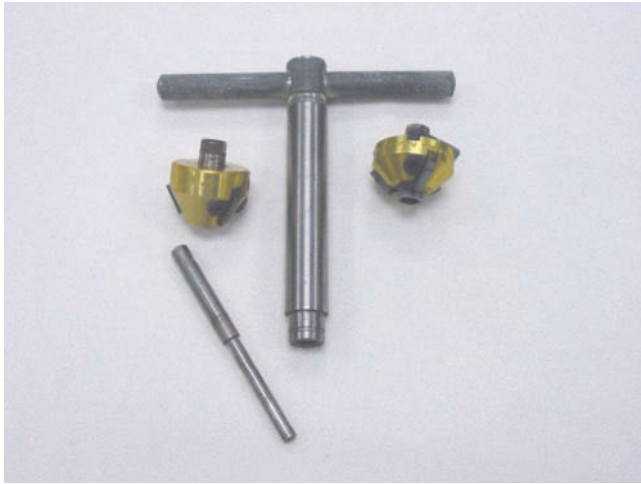
Figure 12-41 A typical valve seat cutting tool with its various components.
