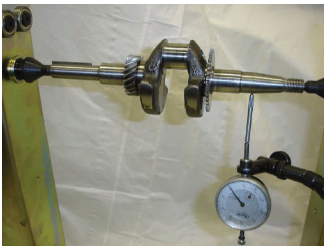
Figure 12-87 Measuring a crankshaft to make sure it's not bent, by checking for run out.
