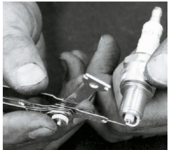
Figure 16-21 Measuring spark plug end gap using a wired-end spark plug gap tool.
