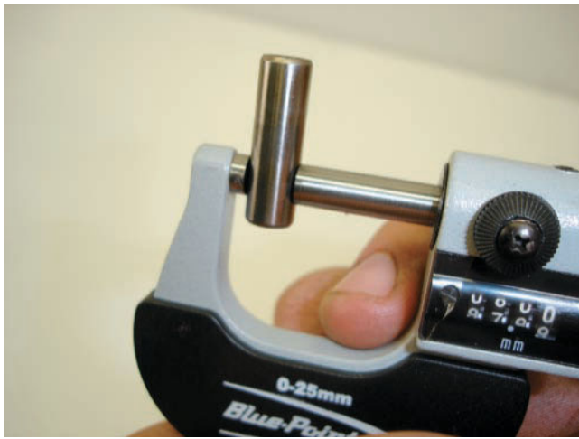
Figure 10-25 Measuring the wrist pin.
