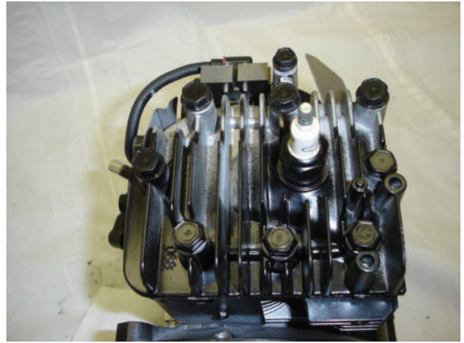
Figure 12-10 A close-up of the L-head attached to the engine.
