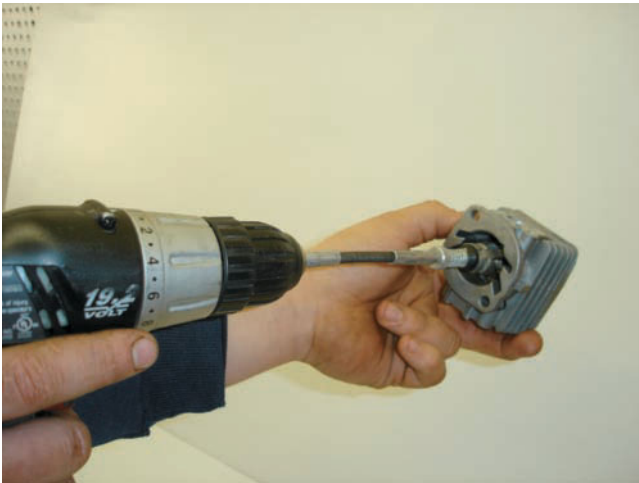
Figure 10-22 Deglazing a cylinder provides the best seal and quick break-in when replacing a piston and/or piston ring.
