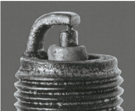
Figure 16-19 A bridged gap is caused by carbon or oil deposit buildup in the spark plug electrode gap until the gap is closed. Courtesy of Federal-Mogul Corporation.
