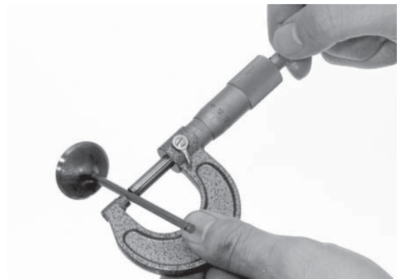
Figure 12-29 A micrometer is used to measure the valve stem. Copyright by American Honda Motor Co., Inc. and reprinted with permission.
