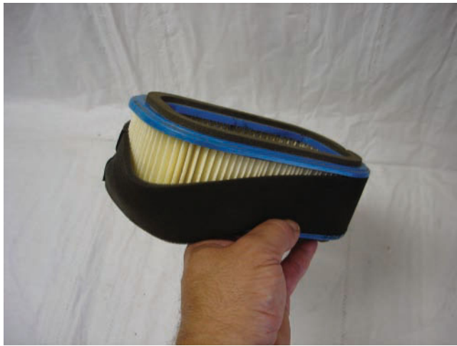
Figure 16-39 In some cases, foam filters are used in conjunction with paper air filters as a pre-filtering device.
