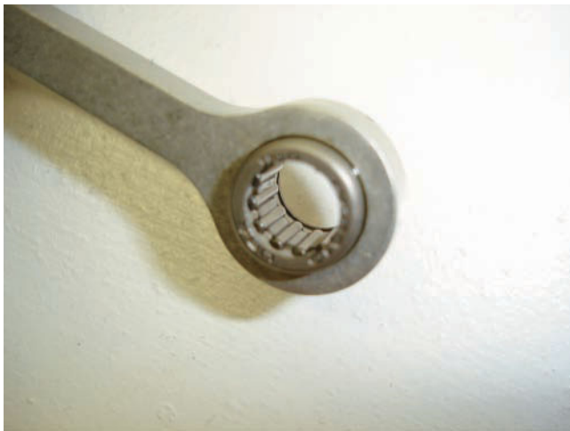
Figure 10-26 The two-stroke engine rod will usually use a bushing or needle bearing at the small end.
