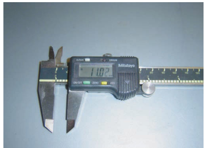
Figure 3-48 Some people feel that reading a digital caliper is easier than reading the standard vernier scale. As you can see here, that point is hard to argue!
