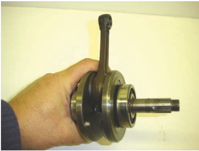
Figure 11-16 A multi-piece crankshaft is often rebuildable.
