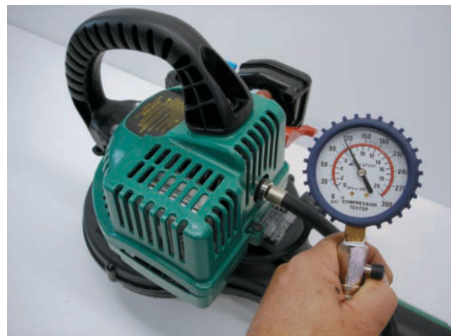
Figure 10-2 A compression check is a simple test that measures the amount of pressure produced in the combustion chamber in the compression stroke.
