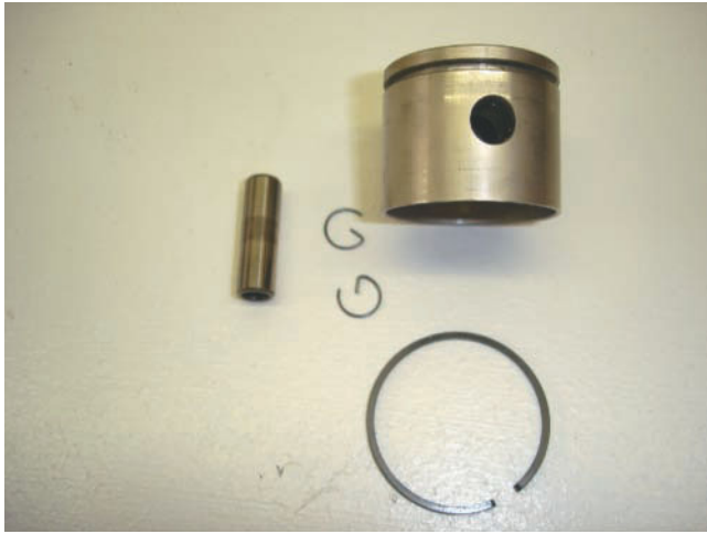
Figure 10-11 The piston assembly consists of the piston wrist pin, clips, and the piston ring.
