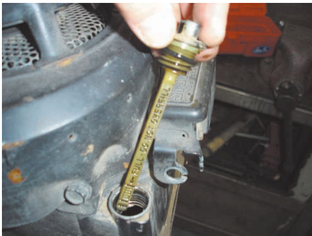
Figure 16-6 Generally speaking, the most popular method of checking the oil level in power equipment engines is by use of a screw-in dip-stick.
