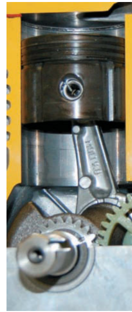
Figure 5-18 Piston rings are located in the slots on the outside diameter of the piston to make a seal between the piston and cylinder wall. The piston travels up and down in the cylinder, as shown in this cutaway.
