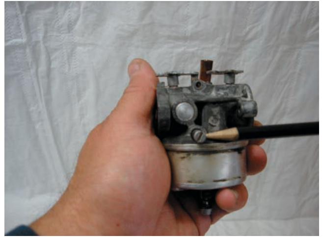
Figure 8-11 A low-speed adjustment screw is typically on the side of the carburetor, as seen here.
