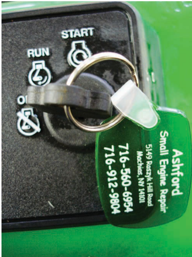
Figure 14-55 A properly working key switch will show a complete connection in one position and an open connection in the other.
