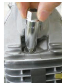
Figure 16-15 A spark-plug socket is a special socket wrench that's specifically designed for removing and installing spark plugs.
