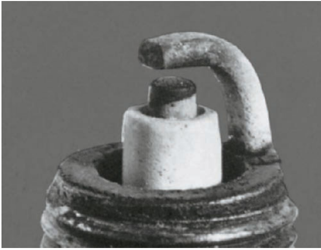
Figure 16-16 A spark plug in normal condition. Note that the bottom surface of the center electrode is flat and the surfaces of the lower electrode are squared. Courtesy of Federal-Mogul Corporation.
