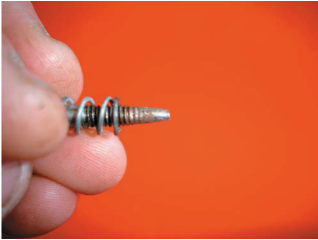
Figure 8-10 The high-speed mixture screw has a taper in it to adjust the flow of fuel in through the carburetor.
