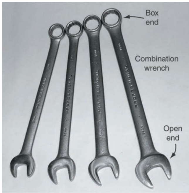
Figure 3-9 Combination wrenches are among the most popular wrenches found in a power equipment engine technician's toolbox.
