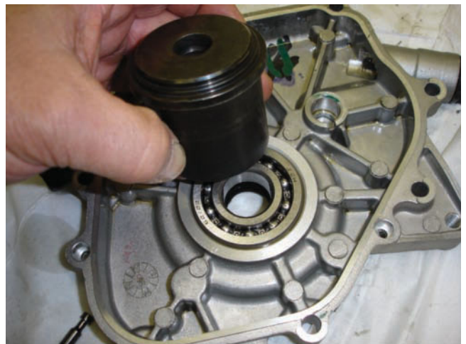
Figure 12-81 Using a special bearing-driver tool to install a new ball bearing will ensure that you do not damage the new bearing during installation.
