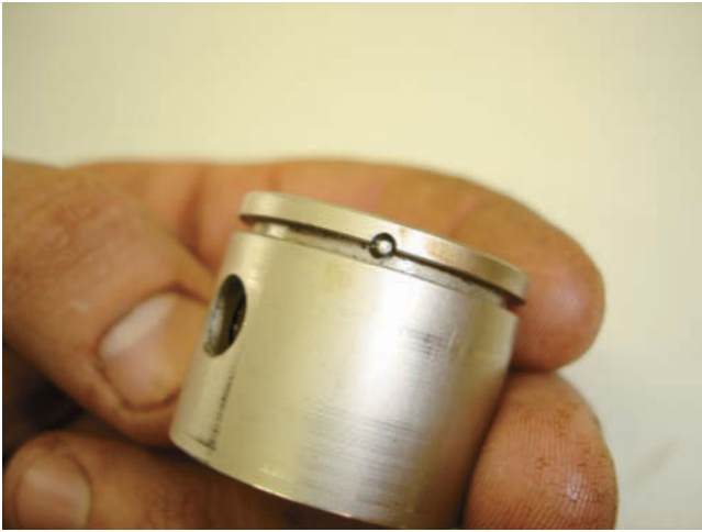
Figure 10-21 Locating pins prevent the piston ring from moving into a port and causing damage in a two-stroke engine.
