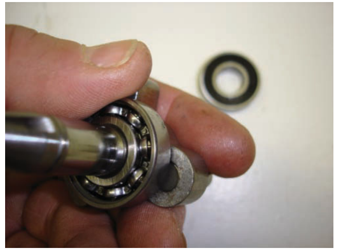
Figure 11-11 Ball bearings are the most common bearing found in a two-stroke engine and are easy to inspect for wear or damage.
