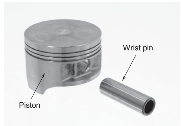
Figure 12-69 The piston wrist pin is used to link the piston to the connecting rod and is also a bearing surface that requires inspection and measurement. Copyright by American Honda Motor Co., Inc. and reprinted with permission.
