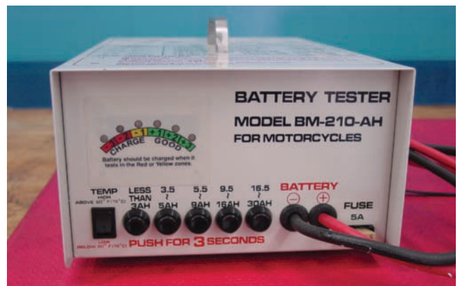
Figure 14-46 Load testers are used to test a battery's ability to withstand high electrical loads. This particular unit shows that it's for motorcycles but is used on any type of battery that fits within its range.
