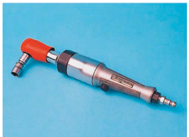
Figure 3-42 An air ratchet can aid in the speed of removal of fasteners, but should not be used to tighten fasteners.
