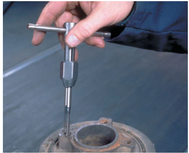
Figure 4-28 A technician chasing threads with a tap.
