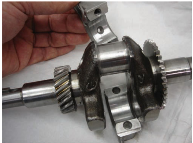
Figure 12-76 The bearing surface on connecting rods found in the typical four-stroke power equipment engine is of the plain bearing design.
