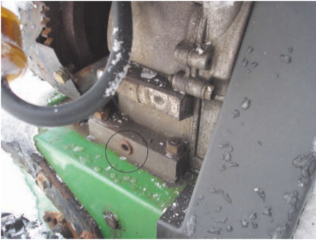
Figure 16-1 The drain plug for a four-stroke engine is generally at the bottom of the engine crankcase.
