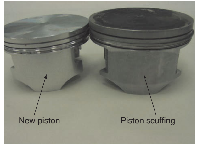
Figure 12-57 The piston on the left is new, whereas the piston on the right has signs of scuffing caused by dirt ingestion through the air-filtering system.
