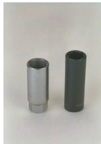
Figure 3-15 You can easily tell the difference between hand and impact sockets. The impact socket is black in color and the hand socket is chrome plated.
