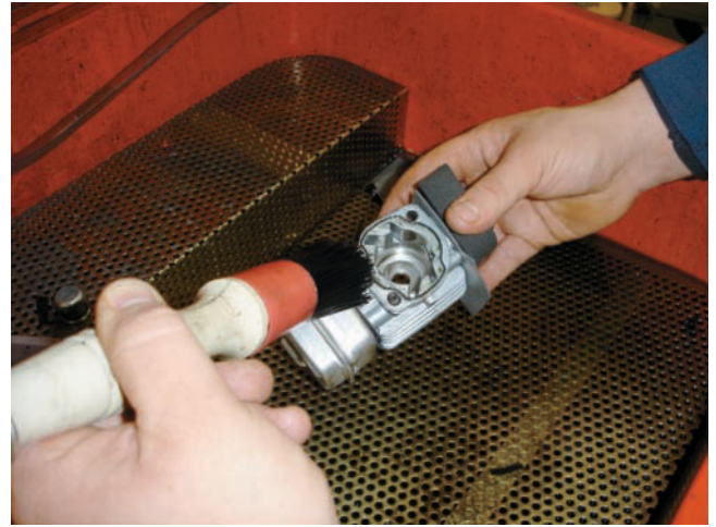
Figure 10-5 Careful cleaning of all the components is an important part of the disassembly process.
