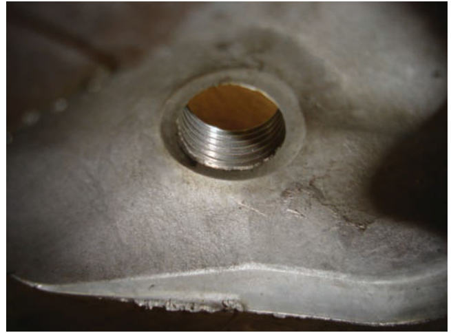
Figure 12-16 The most common problem found on cylinder heads is a stripped spark plug hole. This is something that can be easily repaired when proper tools are used.
