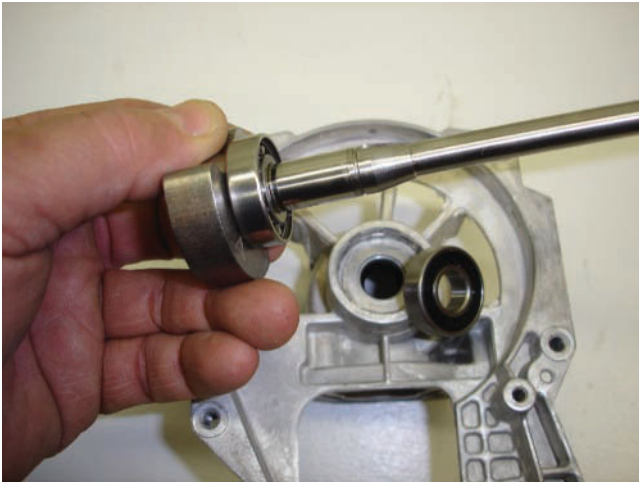
Figure 11-13 Ball bearings must be driven out of the crankcase or pulled off the shaft it's installed on.
