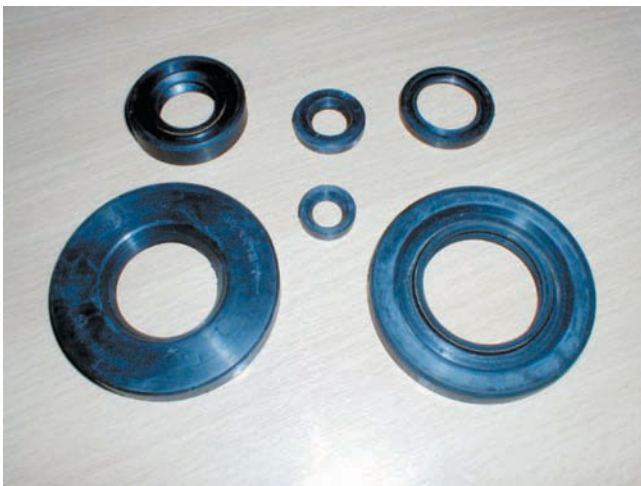
Figure 5-14 Seals used in engines protect the rotating shafts and seal in lubricants and prevent outside contaminants from getting into the engine.
