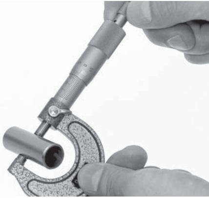
Figure 12-70 Measuring a piston pin with an outside micrometer. Copyright by American Honda Motor Co., Inc. and reprinted with permission.
