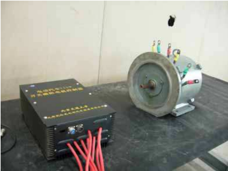
Fig. 23. SR drive system for EV
