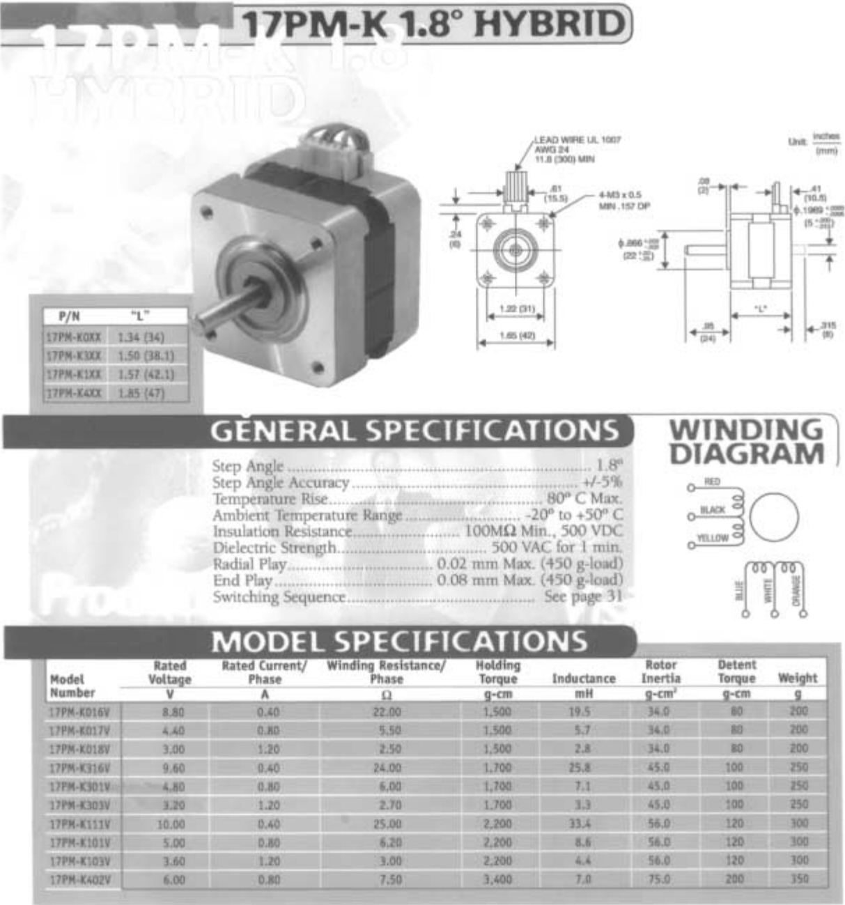
Figure 8.18 Hybrid stepper motors. (Courtesy of NMB Corp.)
