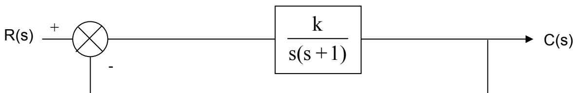
$$\begin{cases} r(t) = 0.2t \\ R_{(s)} = \frac{0.2}{s^2} \Rightarrow C_{ss} = \lim_{s \rightarrow 0} \frac{sR_{(s)}}{1 + G_{(s)} H_{(s)}} = \lim_{s \rightarrow 0} \frac{0.2}{s + \frac{k}{s+1}} \\ H_{(s)} = I \end{cases}$$
