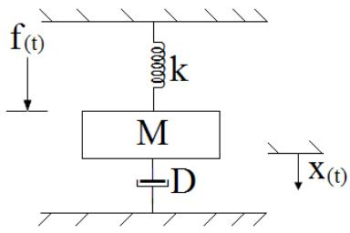
$$\begin{aligned} f_{(t)} &= M \ddot{x} + D \dot{x} + kx \\ f_{(s)} &= s^2 M x_{(s)} + s D x_{(s)} + k x_{(s)} \\ f_{(s)} &= (s^2 M + s D + k) x_{(s)} \end{aligned}$$
