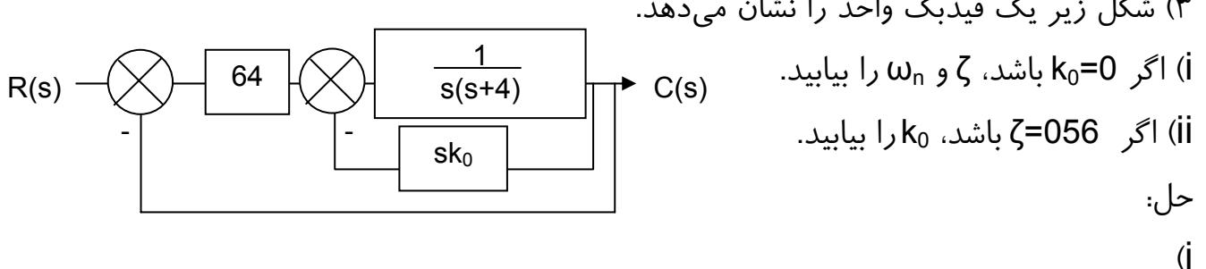
$$G(s) = \frac{64}{s(s + 4) + 64} = \frac{64}{s^2 + 4s + 64} \left\{ \begin{array}{l} \omega_n = 8 \\ 2\zeta\omega_n = 4 \end{array} \right. \Rightarrow \boxed{\zeta = \frac{1}{4} = 0.25}$$
