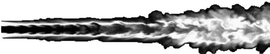
Figure 1.7 Transition from a laminar to a turbulent jet via computer simulation. The regular pattern of disturbances at the left evolves into the disorderly pattern at the right. Courtesy of B. J. Boersma.
