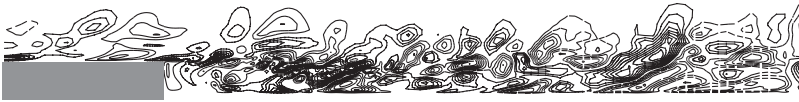
Figure 13.9 Contours of spanwise velocity in flow over a backstep using the SAS model. Courtesy of Dr. Jongwook Joo.
