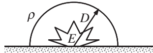
FIGURE 1.11 In an atmosphere with undisturbed density \rho , a point release of energy E produces a hemispherical blast wave that travels a distance D in time t .
