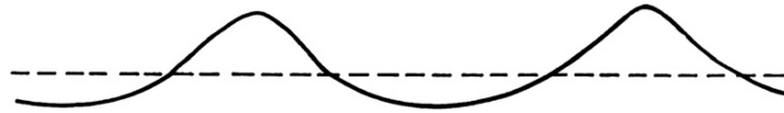
FIGURE 7.21 The waveform of a Stokes wave. Stokes waves are finite-amplitude, periodic irrotational waves in deep water with crests that are more pointed and troughs that are broader than sinusoidal waves.
