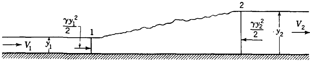
FIG. 11.4. Hydraulic jump in horizontal rectangular channel.
