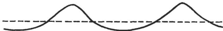
Figure 7.24 The Stokes wave. It is a finite amplitude periodic irrotational wave in deep water.
