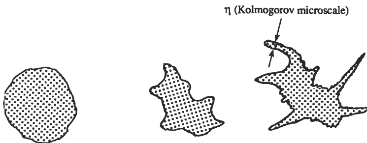
Figure 13.11 Successive deformations of a marked fluid element. Diffusive effects cause smearing when the scale becomes of the order of the Kolmogorov microscale.
