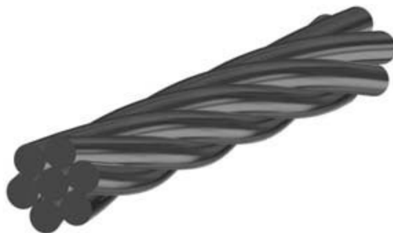
Figure 7.3 Spiral seven-wire strand.
