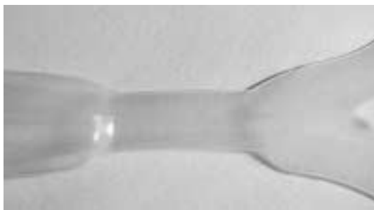
Figure 7: Necking and drawing in a 6-pack holder.
