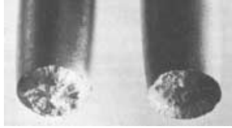
Figure 5: Cup-and-cone fracture in a ductile metal.
