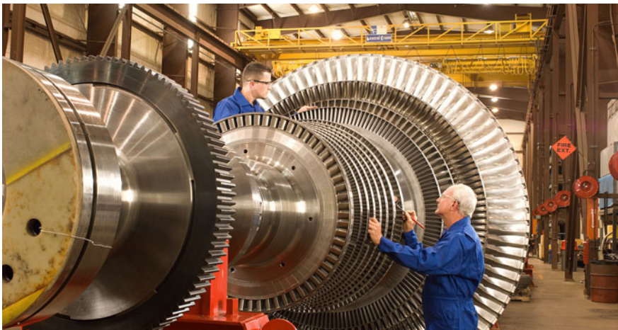
Fig. 5.18: The rotor of a power generation steam turbine. The first four stages of the high pressure part with a constant diameter are followed by intermediate and low pressure stages with increasing blade heights and mean diameters.
