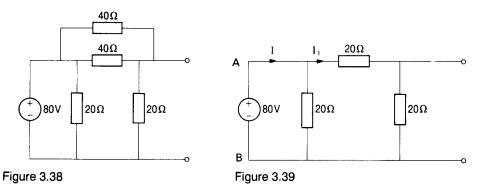
The equivalent resistance between the terminals A and B in Fig. 3.39 is given by
