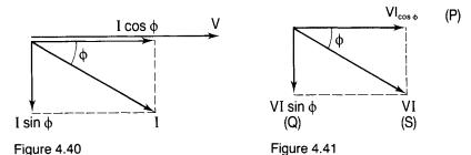
currents by V we obtain the phasor diagram of Fig. 4.41 and, in this diagram: VI is a phasor representing the so-called apparent power (symbol S) which is measured in volt-amperes (VA);  $VI \cos \phi$  is a phasor representing the real power (symbol P) which is measured in watts (W); and  $VI \sin \phi$  is a phasor representing the reactive power (symbol Q) which is measured in volt-amperes reactive (Var).
