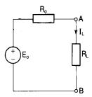
• Step 3: to calculate  $E_0$  remove the resistor  $R_L$  in Fig. 3.14 to give the circuit of Fig. 3.16 and determine the potential difference between the terminals A and B (say  $V_{AB}$ ).
