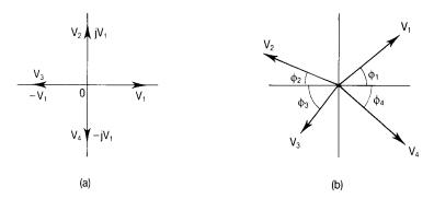
The phasor  $V_3$  has the same length as  $V_2$  but is 90° ahead of it so that  $V_3 = jV_2$ . But from equation (4.19)  $V_2 = jV_1$ , so
