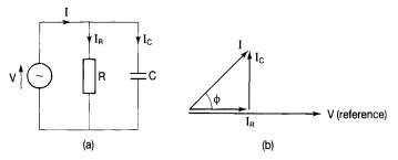
The magnitude of I is thus  $\sqrt{[(I_R^2 + I_C^2)]}$  and the phase angle  $\phi$  is  $\tan^{-1}$   $(I_C/I_R)$ . Since I = V/Z,  $I_R = V/R$  and  $I_C = V/X_C$  we have
