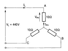
1 The voltage across each resistor is the phase voltage, and from Equation (5.1)
