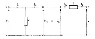
We saw in Example 9.7 that for a shunt admittance A = 1, B = 0, C = Y and D = 1. Also, from Example 9.4 we have, for series impedance, A = 1, B = Z, C = 0 and D = 1.
