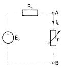
and B at either end of the resistor, r. To calculate  $E_0$  we first remove the resistor r in the circuit of Fig. 3.18 to give the circuit of Fig. 3.20.
