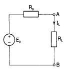
load resistor  $R_{\rm L}$  is given by  $P_{\rm L} = I_{\rm L}^2 R_{\rm L}$ . But  $I_{\rm L} = E_0 / (R_0 + R_{\rm L})$  so that
