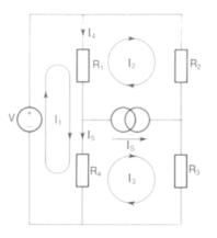
Applying KVL to mesh 1 and taking the clockwise direction to be positive, we have
