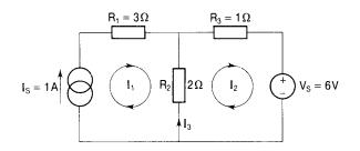
There are two meshes whose currents are  $I_1$  and  $I_2$ , respectively, and we note that the mesh current  $I_1$  is equal to the current source  $I_5$ . Applying KVL to mesh 2 and taking the anticlockwise direction to be positive, we have
