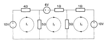
13 Determine the current *I* supplied by the voltage source in the circuit of Fig. 7.20.
