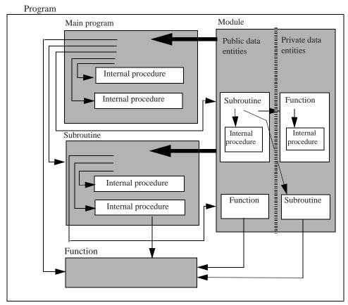
Figure 2-1 Example of program packaging. The thick arrows represent use association; the thin arrows represent procedure references.
