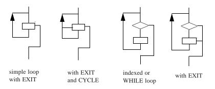
Figure 8-4 Execution flow for DO constructs
