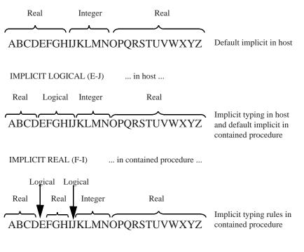
Figure 16-3 How the mapping of implicit typing progresses from host to contained procedure
