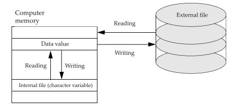
Figure 9-5 External and internal files
