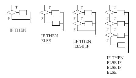
Figure 8-1 Execution flow for IF constructs.
