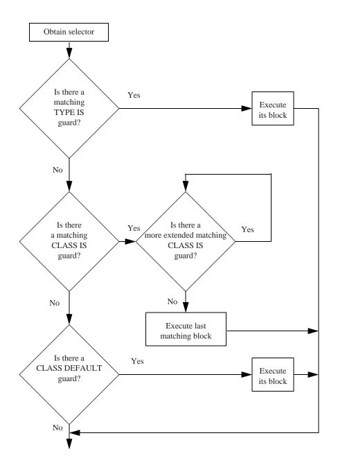
**Figure 8-3** Block selection process for a SELECT TYPE construct. A TYPE IS guard matches if the dynamic type and type parameters values of the selector match the guard. A CLASS IS guard matches if the dynamic type of the selector is an extension of the type of the guard and the kind type parameter values match.
