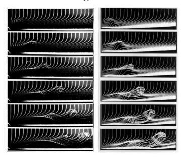
**Fig. 1.10.** Comparison of hydrogen bubble flow visualizations (*left*) of incompressible flat plate boundary-layer transition with DNS results of Zang, Hussaini and Erlebacher (*right*) [Reprinted with permission from T.A. Zang, M.Y. Hussaini (1987); © 1987 ASME]
