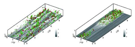
Fig. 1.11. Turbulent fluctuations near the bottom wall in incompressible pulsating channel flow from the LES computations of Scotti and Piomelli (2001). The left frame is near the end of the acceleration phase and the right frame is at the middle of the deceleration phase of the cycle [Reprinted with permission from A. Scotti, U. Piomelli (2001); © 2001, American Institute of Physics]
