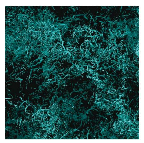
Fig. 1.6. Direct numerical simulation of incompressible isotropic turbulence on a 2048<sup>3</sup> grid by Y. Kaneda and T. Ishihara (2006): High-Resolution Direct Numerical Simulation of Turbulence. Journal of Turbulence 7(20), 1–17. The figure shows the regions of intense vorticity in a subdomain with 1/4 the length in each coordinate direction of the full domain [Reprinted with kind permission by the authors and the publisher Taylor & Francis Ltd., http://www.tandf.co.uk/journals]
