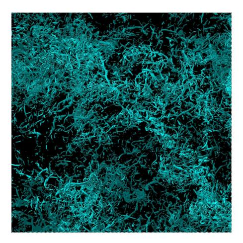
**Fig. 1.6.** Direct numerical simulation of incompressible isotropic turbulence by Kaneda and Ishihara (2006) on a 2048<sup>3</sup> grid. The figure shows the regions of intense vorticity in a subdomain with 1/4 the length in each coordinate direction of the full domain [Reprinted with kind permission by the authors]
