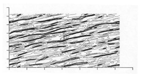
Fig. 1.7. Two-dimensional slice illustrating contours of the pressure field from a compressible homogeneous turbulence DNS by Blaisdell and Zeman (1992) [Reprinted with permission from G.A. Blaisdell, O. Zeman (1992); Center for Turbulence Research, Stanford University/NASA Ames Research Center]
