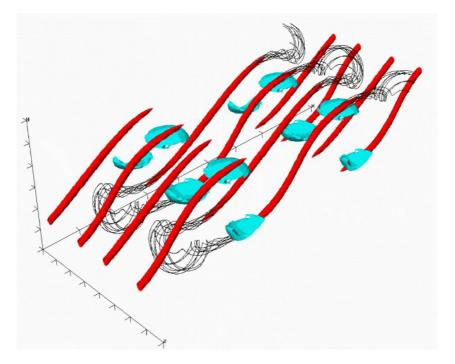
**Fig. 1.9.** DNS of vortex rollup in an incompressible free shear layer by Rogers and Moser (1992). The surfaces denote two types of regions of strong vorticity and the lines are vortex lines [Reprinted with permission from M.M. Rogers, R.D. Moser (1992); © 1992, Cambridge University Press]
