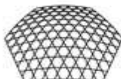
(i) Three-way grid dome
