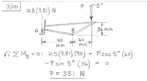
Assumptions: The weight of the panel acts at the 90-mm dimension as shown above; panel does not slip.
