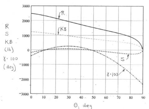
$R_{\text{max}} = 2490 \text{ 16 @ } \theta = 0$   $|S|_{\text{max}} = 259 \text{ 16 @ } \theta = 81.6^{\circ}$
