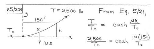
Numerical or graphical (see below) solution:  $T_0 = 1863$  lb. Then Eq. 5/22:  $T = T_0 + \mu h$ : 2500 = 1863 + 10h, h = 63.7 ft 5/22:  $S = 2s = 2\frac{T_0}{\mu} \sinh \frac{\mu x}{T_0}$  $= 2\frac{1863}{10} \sinh \frac{10(150)}{1863} = 333$  ft
