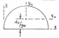
$$I_{xy} = I_{x_0y_0} + Ad_{x_0dy} = 0 + \frac{\pi r^2}{2} (r) (\frac{4r}{3\pi}) = \frac{2}{3} r^4$$
