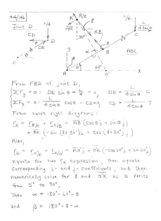
From FBD of ABC:  $A = 0: -\frac{L}{4}(\overline{Ac} \cos \theta) - \frac{L}{4 \tan \theta}(\overline{Ac} \sin \theta)$ + KB cos ( $\beta$ - $\theta$ ) ( $\overline{AB}$  sin  $\theta$ ) + K8 sin ( $\beta$ - $\theta$ ) ( $\overline{AB}$  cos  $\theta$ ) = 0 Solve this for force KB. From the final FBD  $\frac{R}{2}$  - KB cos  $\delta$  = 0  $\Rightarrow$  Gives R  $\frac{S}{2}$  - KB sin  $\delta$  = 0  $\Rightarrow$  Gives S' For L= 800 16, Ao' = 8.75", AB = 8", BK = 9" and
