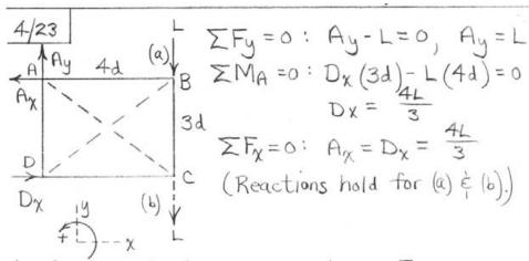
(a) Assume that BD goes slack. From an inspection of joint B, AB=0 and BC=L C. Similarly, from joint D, AD=0 and  $CD=\frac{4L}{3}$  C.
