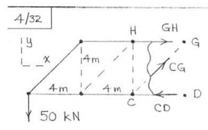
$\Sigma F_y = 0$ :  $CG \sin 45^\circ - 50 = 0$ , CG = 70.7 kN T  $\Sigma M_c = 0$ : GH(4) - 50(8) = 0, GH = 100 kN TAll members except EF are statically determinate, iso above solution is unaffected by the redundant support.
