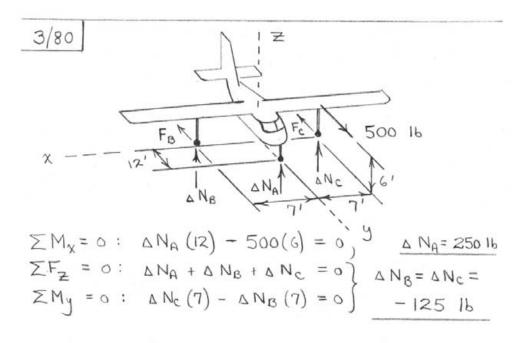
More information would be required to determine FB and Fc. X-components of friction at B and C are possible.
