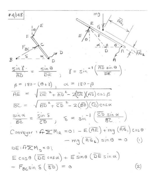
Solve Eqs. (1) 4 (2) for E and FBC as functions of  $\Theta$  for the values  $\overline{AD}=1060$  mm,  $\overline{DE}=1945$  mm,  $\overline{CD}=1150$  mm,  $\overline{AG}_1=2130$  mm,  $\overline{AG}_2=500$  mm, and  $\overline{MG}_3=100$  (9.81) N to obtain the following plot:
