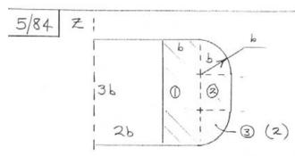
$$V_{1} = 2\pi \, \overline{r}_{1} \, A_{1} = 2\pi \, \left(2b + \frac{b}{2}\right) (3b^{2}) = 15\pi b^{3}$$
