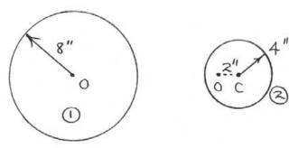
Area  $A = A_1 - A_2 = \pi (8^2 - 4^2) = 48\pi \text{ in.}^2$ ①  $I_{0_1} = \frac{1}{2} (\pi 8^2) 8^2 = 2048\pi \text{ in.}^4$ ②  $I_{0_2} = +\frac{1}{2} (\pi 4^2) 4^2 + \pi (4)^2 (2^2) = +192\pi \text{ in.}^4$ So  $I_0 = I_{0_1} - I_{0_2} = 1856\pi \text{ in.}^4$   $k_0 = \sqrt{\frac{1856\pi}{48\pi}} = 6.22 \text{ in.}$
