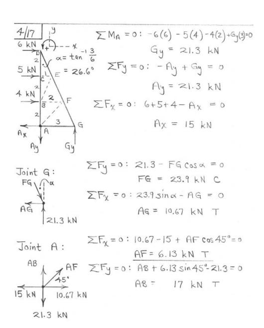
Joint F:  $\sum F_y = 0$ :  $-EF\cos \alpha + 23.9\cos \alpha$  = F  $-6.13\sin 45^\circ = 0$ , EF = 19.01 kNC  $= 25^\circ$   $= 25^\circ$  = 25
