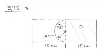
$$V_{1} = 2\pi r_{1} A_{1} = 2\pi \left(15 + \frac{15}{2}\right) \left(15 \cdot 10\right) = 21 200 \text{ mm}^{3}$$
