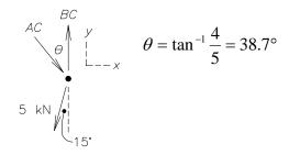
$$\begin{cases} \Sigma F_x = 0: -5\sin 15^\circ + AC\sin 38.7^\circ = 0, \underline{AC} = 2.07 \text{ kN } C \\ \Sigma F_y = 0: BC - 5\cos 15^\circ - 2.07\cos 38.7^\circ = 0, \underline{BC} = 6.45 \text{ kN } T \end{cases}$$
