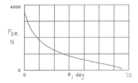
$(F_{DE})_{max} = 3580 \text{ N} @ \Theta = 0$   $(F_{DE})_{min} = 0 @ \Theta_{max} = 65.9^{\circ} \text{ (links AB)}$ and BC are collinear and serve as (an unstable!) prop for the door)
