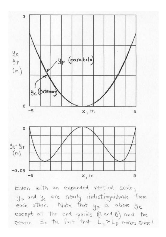
5/167 From Eq. 5/19 with  $\chi = 100 \, \text{m}$ ,  $y = 32 \, \text{m}$   $32 = \left(\frac{70}{\mu}\right) \left[\cosh\left(\frac{100 \, \mu}{T_n}\right) - 1\right]$ Solve by computer or graphically  $4 \, \text{get} \, \frac{16}{\mu} = 161.3 \, \text{m}$ From Eq. 5/22,  $60 \, (10^3) = 7_0 + 32 \, \mu$ Solve Simultaneously  $4 \, \text{get} \, \mu = 310 \, \text{N/m}$ Thus  $P = \frac{\mu}{9} - Pcoide = \frac{310}{9.81} - 18.2 = 13.44 \, \text{kg/m}$  of ice
