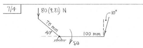
For a virtual displacement 80 of the lever, SU=0:  $P\cos 10^{\circ}(100 80)-80(9.81)[75 80 \cos 40^{\circ}]=0$  P=458 N
