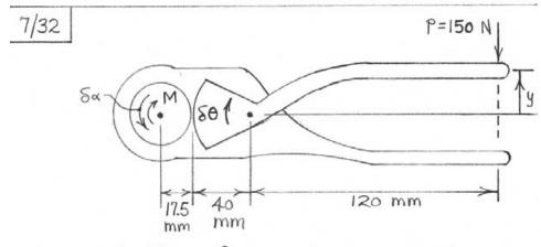
$\delta \alpha = \text{rotation of socket on bolt head}$   $\delta \theta = \text{rotation of upper handle (lower handle}$ and frame taken as fixed)
