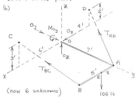
$$T_{AD} = T_{AD} \left[ \frac{-4\underline{i} - 7\underline{i} + 2\underline{k}}{\sqrt{69}} \right]$$
