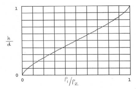
For pine wood and salt water,  $f_1 = 480 \frac{kg}{m^3}$  and  $f_2 = 1030 \frac{kg}{m^3}$ . So  $\frac{f_1}{f_2} = \frac{480}{1030} = 0.466$ Numerical solution:  $\frac{h}{d} = 0.473 = r$
