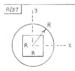
Without square hole:  $I_{Z} = 2I_{X} = 2\left(\frac{1}{4}\pi R^{2} \cdot R^{2}\right) = \underline{1.571R^{4}}$ With hole:  $I_{Z} = 1.571R^{4} - 2\left(\frac{1}{12}R \cdot R^{3}\right) = \underline{1.404R^{4}}$ (a reduction of 10.61%)
