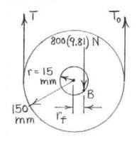
From the solution to  $r_f = 3.64 \text{ mm}$
