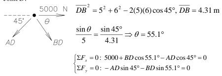
Solve simultaneously to obtain:  $\frac{BD = -3590 \text{ N or } 3590 \text{ N } C}{AD = 4170 \text{ N } T}$
