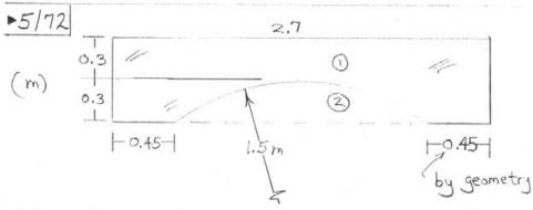
From Prob. 5/41, relative to the base of the current area, we have for the circular portion with a = 1.5 m + 1.2 m:
