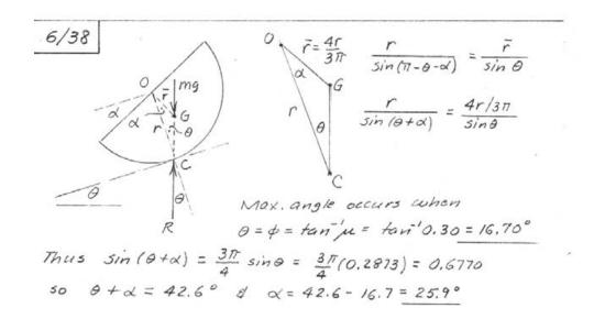
For equilibrium the three forces must be Concurrent at P. For larger than that shown, friction angles & would
