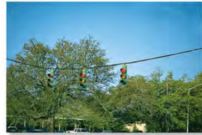
Each of the cable segments remains approximately straight as they support the weight of these traffic lights.
