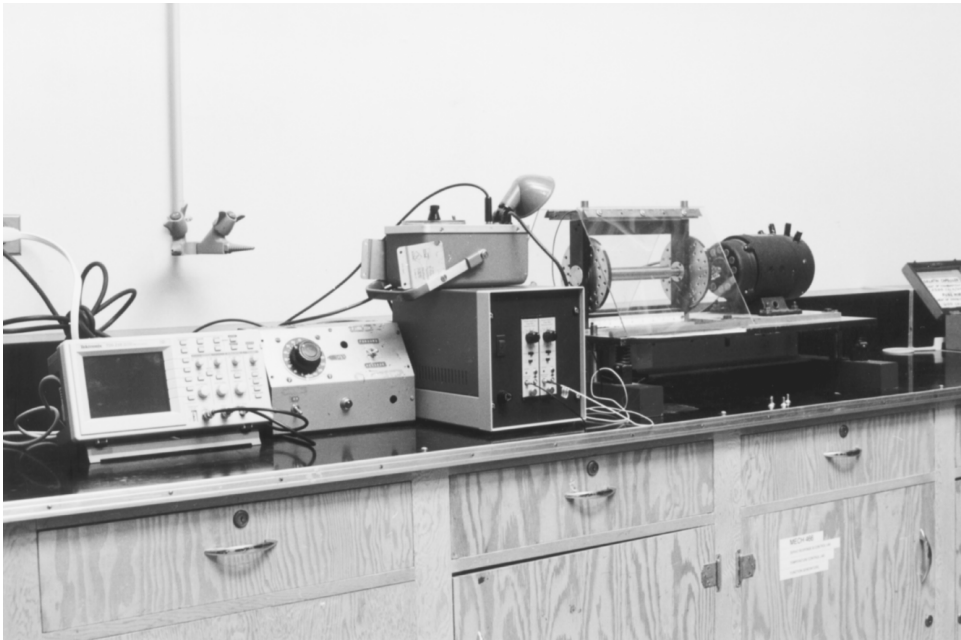
FIGURE 12.15 A view of the experimental setup for two-plane balancing. (Courtesy of the University of British Columbia. With permission.)
