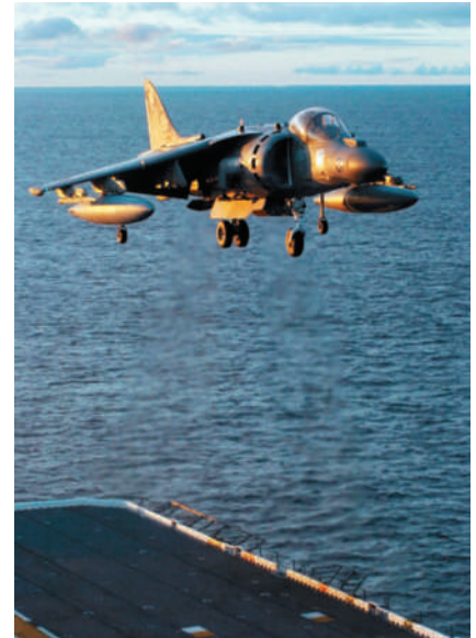
The jet exhaust of this VTOL aircraft can be vectored downward for vertical takeoffs and landings.
