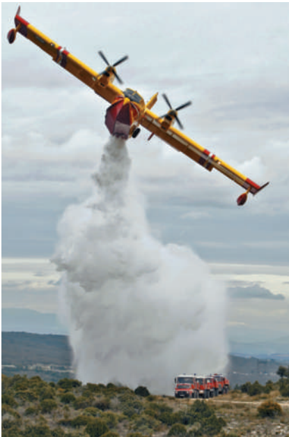
The Super Scooper is a firefighting airplane which can quickly ingest water from a lake by skimming across the surface with just a bottom-mounted scoop entering the water. The mass within the aircraft boundary varies during the scooping operation as well as during the dumping operation shown.
