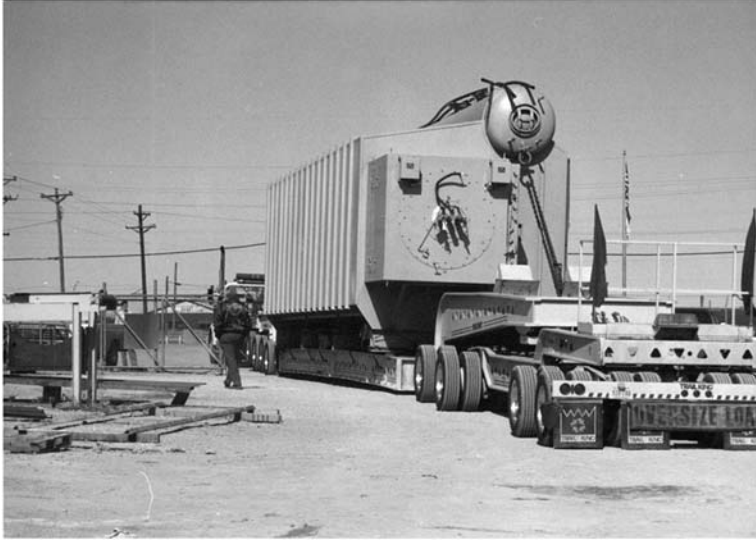
FIGURE 1.5 Packaged steam generator with completely water-cooled furnace. (Courtesy of ABCO Industries, Abilene, TX.)
