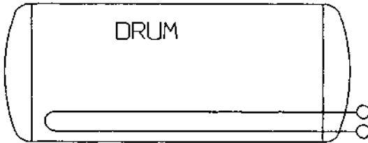
FIGURE 8.12 Exchanger inside boiler drum.
