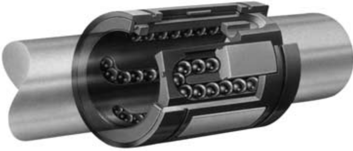
FIGURE 8.3. Linear ball bearing for translating follower (Courtesy Warner Electric, South Beloit, Ill.).
