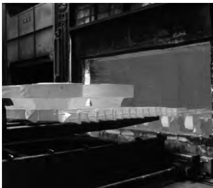
FIGURE 2.38 A large rectangular steel slab as it exits a heat treatment furnace.
