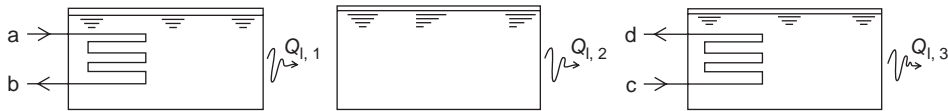
Fig. 9.1. The three stages in a simple heat storage process: charging period (left), storing period (center) and discharging period (right).
