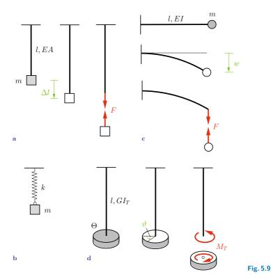
The constant  $k_T$  has the dimensions moment/angle. If a disk (moment of inertia  $\Theta$ ) is fixed to the end of the shaft and undergoes torsional vibrations, then the motion is described by  $\Theta\ddot{\vartheta} + k_T\vartheta = 0$ .
