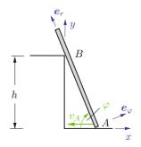
Results: see (B)  $v_B = v_A \cos \varphi \, \boldsymbol{e}_r$ ,  $a_B = \frac{v_A^2}{h} \sin^2 \varphi (-\sin \varphi \, \boldsymbol{e}_r + 2\cos \varphi \, \boldsymbol{e}_\varphi), \quad y = \frac{x^2}{h} + h.$
