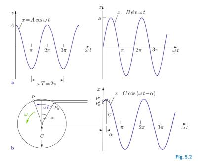
$$x(t) = A\cos\omega t \quad \text{or} \quad x(t) = B\sin\omega t$$
