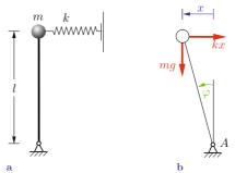
**Solution** We introduce the coordinates  $\varphi$  (positive counterclockwise) and x as shown in Fig. 5.8b. Then the elongation of the spring is given by  $x = l \sin \varphi$ . The principle of angular momentum (1.67) leads to the equation of motion  $(\Theta_A = ml^2)$ :
