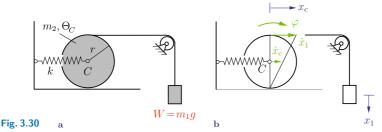
**Solution** We introduce the coordinates  $x_1, x_c$  and  $\varphi$ , measured from the initial position (Fig. 3.30b). In this position, the potential and the kinetic energy are zero:
