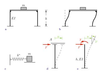
The frame has two columns in parallel. Therefore, the spring constant of the frame is given by  $k^* = 2 k_c$ . Hence, the natural frequency of the system is found to be
