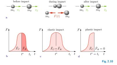
Since the precise time variation of F(t) (Fig. 2.10b) during the impact is usually unknown, we apply the concept of *linear impulse*  $\hat{F}$  as we did in Section 1.2.5. We write down the linear impulse for the compression phase and for the restitution phase, respectively:
