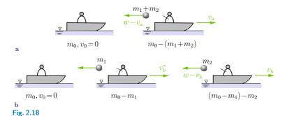
**Solution** Fig. 2.18a shows the situations before and after the ejection of the masses in case a). The ejected mass  $m_1 + m_2$  moves relative to the boat with the velocity w to the left. If the boat moves with the velocity  $v_a$  to the right, then the masses  $m_1 + m_2$  have the absolute velocity  $w - v_a$  to the left. Since the initial momentum is zero  $(v_0 = 0)$ , the principle of conservation of linear
