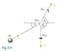
mentum of the system does not change (linear momentum before splitting = linear momentum after splitting). Componentwise, the principle of conservation of linear momentum gives
