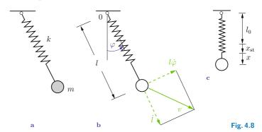
**Solution** The position of the point mass is uniquely determined by its distance l from pin 0 and by the angle  $\varphi$  (Fig. 4.8b). Hence, the system has two degrees of freedom. It is often advantageous to use dimensionless quantities as generalized coordinates; here we
