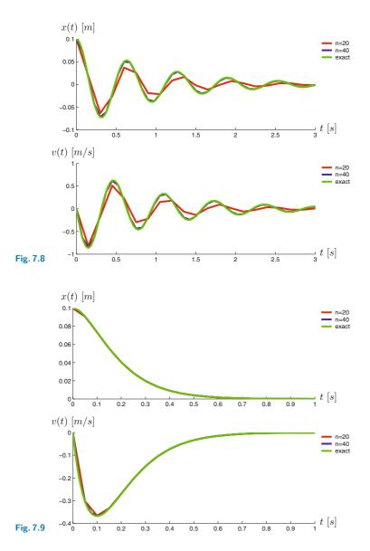
In the fourth example we analyse the vibration of a damped system subjected to a harmonic force and the initial conditions
