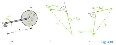
**Solution** We solve the problem with a graphical/analytical method. The center A of the disk moves in a circle about 0. Thus,
