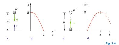
We will now examine the vertical motion of a body that is thrown vertically at time t = 0 from the earth's surface  $(z_0 = 0)$ with initial velocity  $v_0$  (Fig. 1.4c). It follows from (1.10), that
