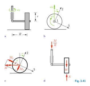
As an illustrative example where this difficulty does not occur, we consider the rolling motion of a wheel in a grinding mill whose vertical king shaft rotates with constant angular velocity  $\omega_0$  (Fig. 3.41a). We assume that the moments of inertia with respect to the wheel-fixed rotating principal axes (see Fig. 3.41b) are known. Furthermore, because the wheel is assumed to be axisymmetric,  $\Theta_2 = \Theta_3$ . From kinematics we obtain
