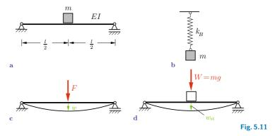
**Solution** We reduce the system consisting of the massless beam and the mass to the equivalent simple system of a spring and a mass (Fig. 5.11b). To determine the equivalent spring constant  $k_B$  we subject the beam to a force F which acts at the location of the box (Fig. 5.11c). This force produces the deflection (see Volume 2)
