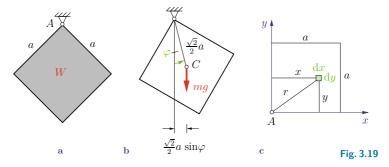
**Solution** The plate rotates about the fixed axis that is perpendicular to the plane of the plate and passes through A. We introduce the angle  $\varphi$  as shown in Fig. 3.19b and apply the principle of angular momentum:
