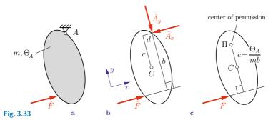
With the velocities  $\bar{v}_x = c \bar{\omega}$  and  $\bar{v}_y = -d \bar{\omega}$  of the center of mass (rotation about the fixed point A) we obtain the impulsive pin reactions
