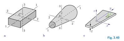
Here,  $I_x$  is the area moment of inertia with respect to the x-axis (cf. Volume 2). Applying this procedure for all components of the inertia tensor, we obtain
