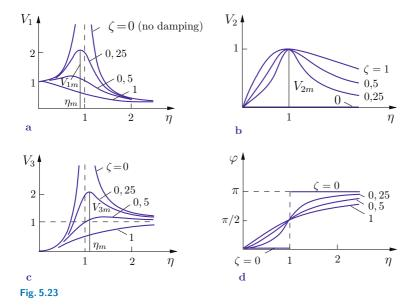
The maximum value  $V_{2m} = 1$  is independent of  $\zeta$  and is always located at  $\eta_m = 1$ .
