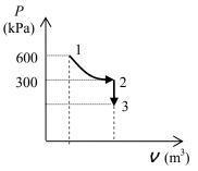
**4-83** Argon at a specified state contained in a piston-cylinder device with a set of stops is compressed at constant temperature until a final volume. The process is to be sketched on the P-V diagram and the amount of heat transfer is to be determined.
