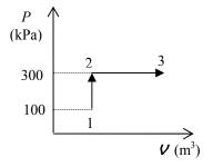
**4-82** Air at a specified state contained in a piston-cylinder device undergoes an isothermal and constant volume process until a final temperature. The process is to be sketched on the P-V diagram and the amount of heat transfer is to be determined.
