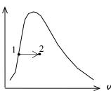
**4-39** A cylinder equipped with an external spring is initially filled with steam at a specified state. Heat is transferred to the steam, and both the temperature and pressure rise. The final temperature, the boundary work done by the steam, and the amount of heat transfer are to be determined, and the process is to be shown on a P-v diagram.
