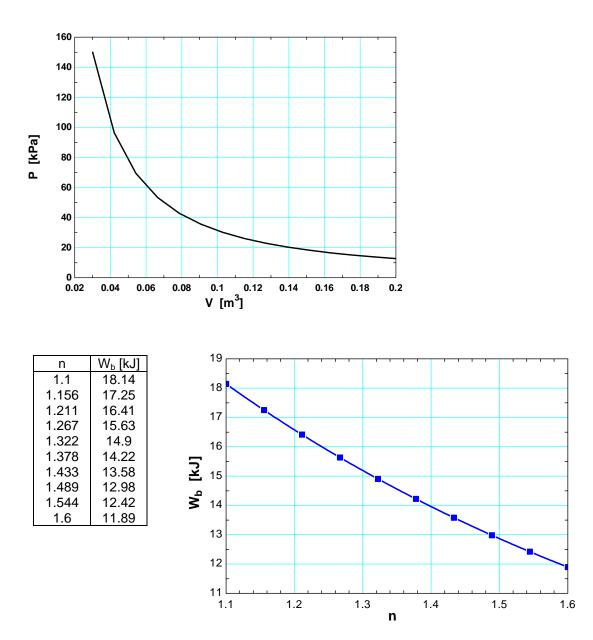
**4-18** Nitrogen gas in a cylinder is compressed polytropically until the temperature rises to a specified value. The boundary work done during this process is to be determined.
