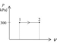
**4-11** Refrigerant-134a in a cylinder is heated at constant pressure until its temperature rises to a specified value. The boundary work done during this process is to be determined.
