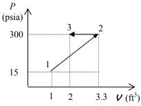
4-6 The work done during the isothermal process shown in the figure is to be determined.
