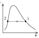
**4-45** Saturated R-134a liquid is contained in an insulated piston-cylinder device. Electrical work is supplied to R-134a. The time required for the refrigerant to turn into saturated vapor and the final temperature are to be determined.
