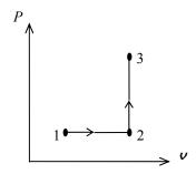
**4-81** Air at a specified state contained in a piston-cylinder device with a set of stops is heated until a final temperature. The amount of heat transfer is to be determined.
