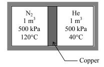
**4-146** Problem 4-145 is reconsidered. The effect of the mass of the copper piston on the final equilibrium temperature as the mass of piston varies from 1 kg to 10 kg is to be investigated. The final temperature is to be plotted against the mass of piston.
