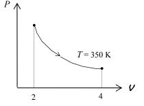
**4-20** Problem 4-19 is reconsidered. Using the integration feature, the work done is to be calculated and compared, and the process is to be plotted on a P - V diagram.
