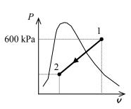
**4-44E** Saturated R-134a vapor is condensed at constant pressure to a saturated liquid in a piston-cylinder device. The heat transfer and the work done are to be determined.
