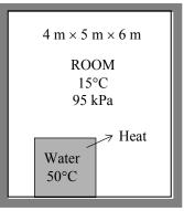
**4-137** A room is to be heated by 1 ton of hot water contained in a tank placed in the room. The minimum initial temperature of the water is to be determined if it to meet the heating requirements of this room for a 24-h period.
