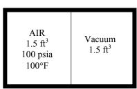
**4-71** Air in a closed system undergoes an isothermal process. The initial volume, the work done, and the heat transfer are to be determined.
