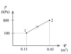
**4-126** A cylinder equipped with a set of stops for the piston is initially filled with saturated liquid-vapor mixture of water a specified pressure. Heat is transferred to the water until the volume increases by 20%. The initial and final temperature, the mass of the liquid when the piston starts moving, and the work done during the process are to be determined, and the process is to be shown on a P-v diagram.
