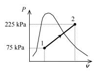
**4-43** R-134a contained in a spring-loaded piston-cylinder device is cooled until the temperature and volume drop to specified values. The heat transfer and the work done are to be determined.
