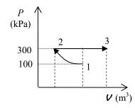
**4-84** An ideal gas at a specified state contained in a piston-cylinder device undergoes an isothermal process during which heat is lost from the gas. The final pressure and volume are to be determined.
