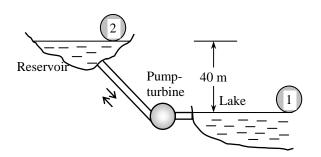
$$W_{\text{max, turbine}} = W_{\text{min, pump}} = W_{\text{ideal}} = \Delta E_{\text{mech}} = \dot{m}\Delta e_{\text{mech}} = \dot{m}\Delta p e = \dot{m}g\Delta z = \rho U_g \Delta z$$
