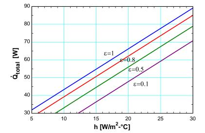
**2-104** Hot air is blown over a flat surface at a specified temperature. The rate of heat transfer from the air to the plate is to be determined.
