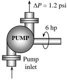
**2-74** Water is pumped from a lower reservoir to a higher reservoir at a specified rate. For a specified shaft power input, the power that is converted to thermal energy is to be determined.
