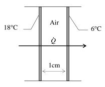
**2-100** Two surfaces of a flat plate are maintained at specified temperatures, and the rate of heat transfer through the plate is measured. The thermal conductivity of the plate material is to be determined.
