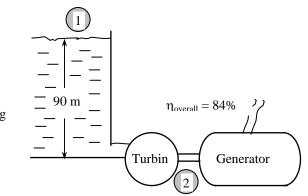
**2-129** An entrepreneur is to build a large reservoir above the lake level, and pump water from the lake to the reservoir at night using cheap power, and let the water flow from the reservoir back to the lake during the day, producing power. The potential revenue this system can generate per year is to be determined.
