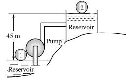
**2-76** A pump is pumping oil at a specified rate. The pressure rise of oil in the pump is measured, and the motor efficiency is specified. The mechanical efficiency of the pump is to be determined.
