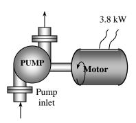
*Discussion* The conservation of energy principle requires the energy to be conserved as it is converted from one form to another, and it does not allow any energy to be created or destroyed during a process. In reality, the volume flow rate will be less because of the losses associated with the conversion of electrical-to-mechanical shaft and mechanical shaft-to-flow energy.
