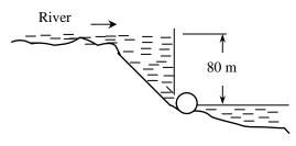
**2-17** A river is flowing at a specified velocity, flow rate, and elevation. The total mechanical energy of the river water per unit mass, and the power generation potential of the entire river are to be determined.
