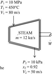
5-53 EES Problem 5-52 is reconsidered. The effect of the turbine exit pressure on the power output of the turbine as the exit pressure varies from 10 kPa to 200 kPa is to be investigated. The power output is to be plotted against the exit pressure.
