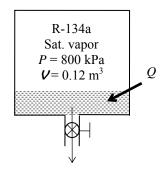
Analysis We take the tank as the system, which is a control volume since mass crosses the boundary. Noting that the microscopic energies of flowing and nonflowing fluids are represented by enthalpy h and internal energy u, respectively, the mass and energy balances for this uniform-flow system can be expressed as
