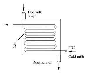
Therefore, to heat the milk from 4 to 72°C as being done currently, heat must be transferred to the milk at a rate of
