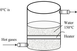
**5-161** Cold water enters a steam generator at 20°C, and leaves as saturated vapor at  $T_{\text{sat}} = 150$ °C. The fraction of heat used to preheat the liquid water from 20°C to saturation temperature of 150°C is to be determined.
