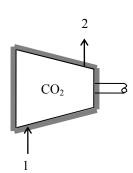
(b) We take the compressor as the system, which is a control volume since mass crosses the boundary. The energy balance for this steady-flow system can be expressed in the rate form as
