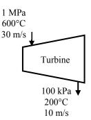
5-50E Air is expanded in a gas turbine. The inlet and outlet mass flow rates are to be determined.
