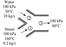
**5-91E** An adiabatic open feedwater heater mixes steam with feedwater. The outlet mass flow rate and the outlet velocity are to be determined for two exit temperatures.
