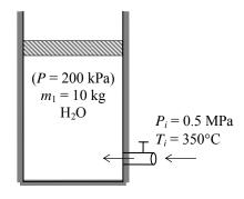
Analysis (a) The cylinder contains saturated vapor at the final state at a pressure of 200 kPa, thus the final temperature in the cylinder must be
