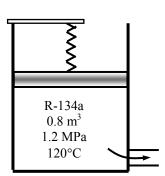
Noting that the spring is linear, the boundary work can be determined from
