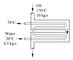
Then the rate of heat transfer to the cold water in this heat exchanger becomes
