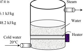
**5-163** Water is boiled at  $T_{\text{sat}} = 100^{\circ}\text{C}$  by an electric heater. The rate of evaporation of water is to be determined.
