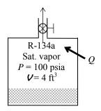
**Analysis** We take the tank as the system, which is a control volume since mass crosses the boundary. Noting that the microscopic energies of flowing and nonflowing fluids are represented by enthalpy h and internal energy u, respectively, the mass and energy balances for this uniform-flow system can be expressed as
