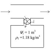
**5-12** A smoking lounge that can accommodate 15 smokers is considered. The required minimum flow rate of air that needs to be supplied to the lounge and the diameter of the duct are to be determined.
