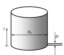
Then the amount of water that flows through the pipe during a differential time interval dt is
