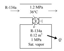
**Analysis** We take the tank as the system, which is a control volume since mass crosses the boundary. Noting that the microscopic energies of flowing and nonflowing fluids are represented by enthalpy h and internal energy u, respectively, the mass and energy balances for this uniform-flow system can be expressed as
