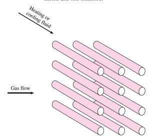
Figure 10-5 | Cross-flow heat exchanger, both fluids unmixed.
