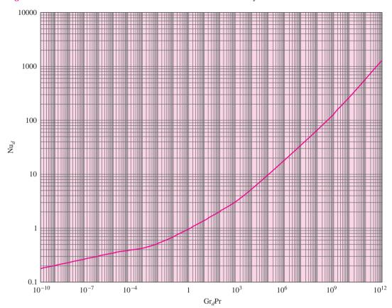
Figure 7-6 | Free-convection heat transfer from horizontal isothermal cylinders.
