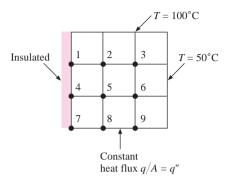
**3-76** Write the nodal equation for nodes 1 through 12 shown in Figure P3-76. Express the equations in a format for Gauss-Seidel iteration.
