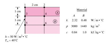
**4-77** Write a nodal equation for analysis of node (m, n) in Figure P4-77 to be used in a transient analysis of the solid.
