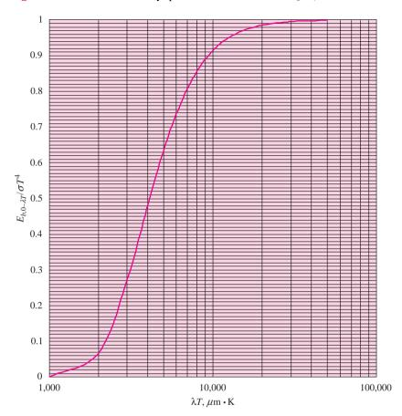
**Figure 12-19** | Planck blackbody spectrum as a function of  $\lambda T$  ( $\mu$ m).
