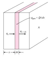
**Figure 1-1** | Sketch showing direction of heat flow.
