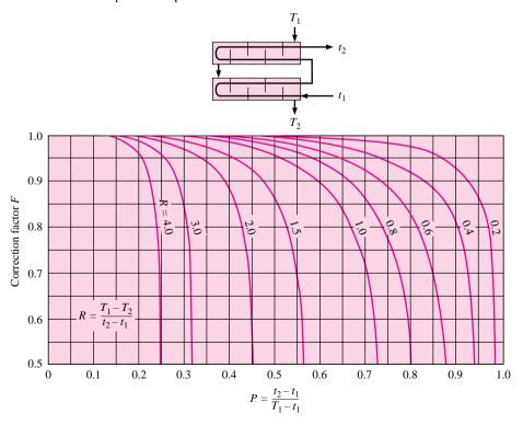
Figure 10-10 | Correction-factor plot for single-pass cross-flow exchanger, both fluids unmixed.
