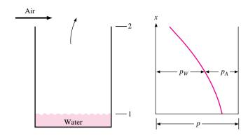
upward with a velocity just large enough to balance the diffusion of air downward. This bulk mass movement then produces an *additional* mass flux of water vapor upward.
