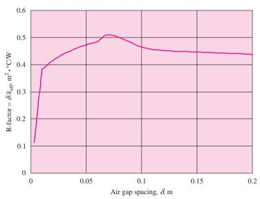
**Figure 12-17** | Free convection across horizontal air gap heated from below at 300 K. See Equation (7-64) and Table 7-3.
