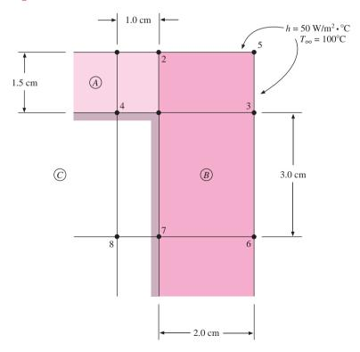
**4-80** Calculate the maximum time increment that can be used for node 5 in Figure P4-80 for a transient numerical analysis. Also write the nodal equation for this node.
