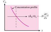
In gases the diffusion rates are clearly dependent on the molecular speed, and consequently we should expect a dependence of the diffusion coefficient on temperature since the temperature indicates the average molecular speed.
