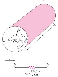
Figure 2-4 | One-dimensional heat flow through multiple cylindrical sections and electrical analog.
