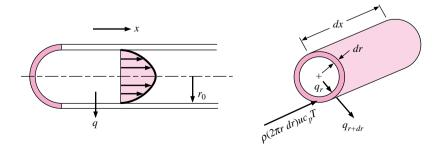
**Figure 5-16** | Force balance on fluid element in tube flow.
