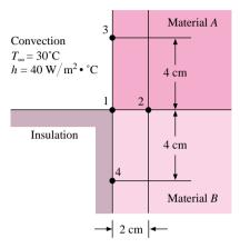
**4-79** Write the transient equation for node 1 in Figure P4-79 and determine the maximum allowable time increment that may be employed in the calculation. The properties of materials *A*, *B*, and *C* are the same as those given in Problem 4-73.
