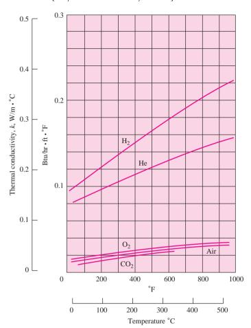
Figure 1-4 | Thermal conductivities of some typical gases  $[1 \text{ W/m} \cdot {}^{\circ}\text{C} = 0.5779 \text{ Btu/h} \cdot \text{ft} \cdot {}^{\circ}\text{F}].$
