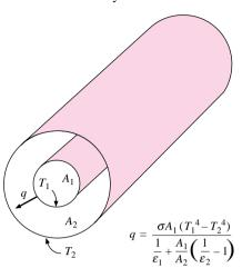
Figure 8-30 | Radiation heat transfer between simple two-body diffuse, gray surfaces. In all cases  $F_{12} = 1.0$ .
