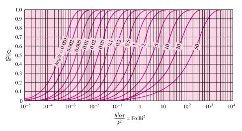
**Figure 4-16** | Dimensionless heat loss  $Q/Q_0$  of a sphere of radius  $r_0$  with time, from Reference 6.
