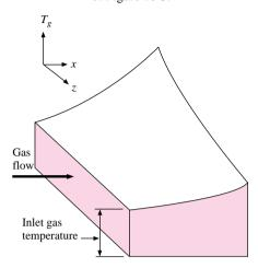
Figure 10-7 | Temperature profiles for (a) parallel flow and (b) counterflow in double-pipe heat exchanger.
