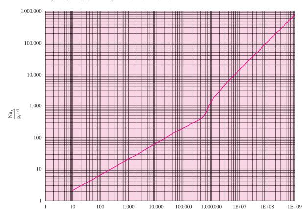
Figure 12-3 | Average Nusselt numbers for flow over isothermal flat plates. Properties evaluated at film temperature  $T_f = (T_w + T_\infty)/2$ . See Equations (5-85) and (5-86).
