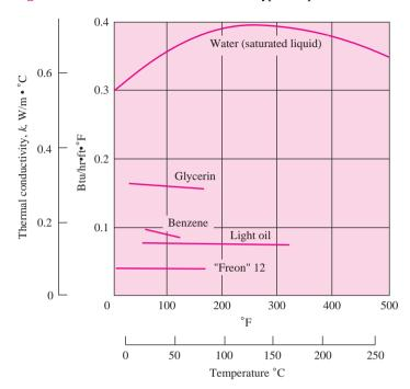
Figure 1-5 | Thermal conductivities of some typical liquids.
