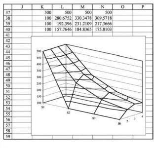
such a block as illustrated in Figure Example D-5(c). For 5 time increments (row 8) the formulas are entered as =\$A8, =\$B8, and so on for nodes 1,2 etc. The fixed boundary temperatures of 100 and 500°C are also entered as constant values for their cell locations. The numerical solutions for  $n = 5\Delta\tau$  then appear in the block of 16 cells.
