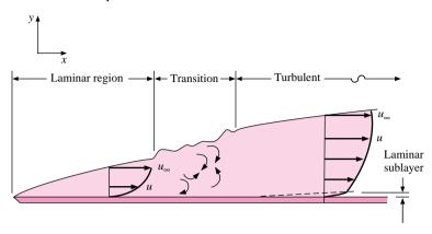
**Figure 5-2** | Laminar velocity profile on a flat plate.
