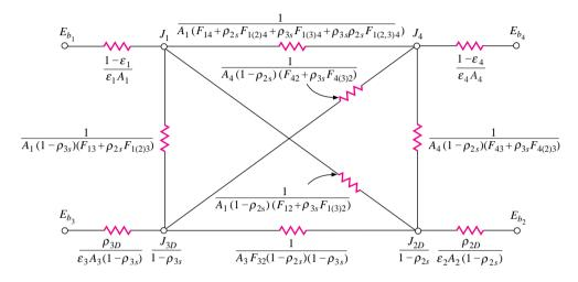
The above two elements are typical for the enclosure of Figure 8-51 and the other elements may be constructed by analogy. Thus the final complete network is given in Figure 8-54.
