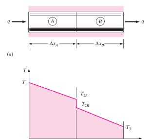
Figure 2-16 | Joint-roughness model for analysis of thermal contact resistance.
