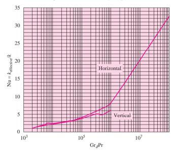
**Figure 12-16** | *R*-factor for free convection across vertical air gap at 1 atm pressure, 300 K,  $\Delta T = 10$  K, L = 0.2 m. See Equation (7-64) and Table 7-3.
