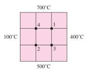
**3-57** Calculate the steady-state temperatures for nodes 1 to 16 in Figure P3-57. Assume symmetry.
