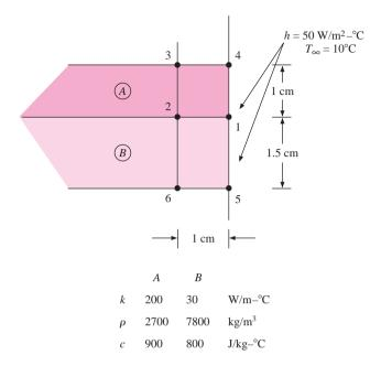
**4-89** Write the nodal equation for a transient analysis of node 2 in Figure P4-89 and determine the stability criterion for this node. The properties for materials *A* and *B* are given in the figure.
