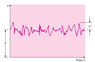
Figure 5-11 | Turbulent fluctuations with time.
