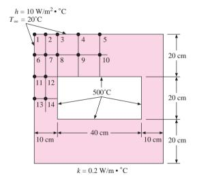
**3-63** Calculate the steady-state temperatures for the nodes indicated in Figure P3-63.
