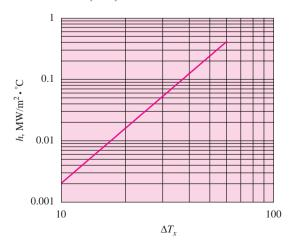
**Figure 12-24** | Approximate boiling heat-transfer coefficients for water at higher pressures (0.7 . See Equation (9-36).
