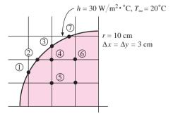
**3-78** Taking Figure P3-78 as a special case of Table 3-2(f), write the nodal equations for nodes (m, n) and 2 for the case of  $\Delta x = \Delta y$ .
