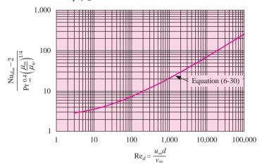
Figure 12-8 | Average Nusselt numbers for free convection from isothermal vertical flat plates. Properties evaluated at film temperature  $T_f = (T_w + T_\infty)/2$ .
