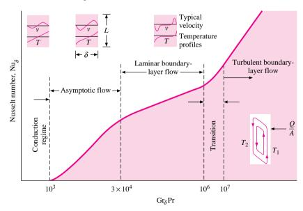
Figure 7-8 | Nomenclature for free convection in enclosed vertical spaces.
