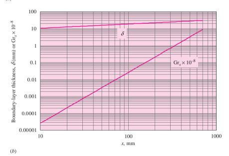
Figure 12-12 | Free-convection boundary-layer thickness on vertical flat plate, x = distance from leading edge, liquid water, properties evaluated at 300 K,  $T_w - T_\infty = 20^{\circ}\text{C}$ : (a) linear plot, (b) log plot. See Equation (7-20a).
