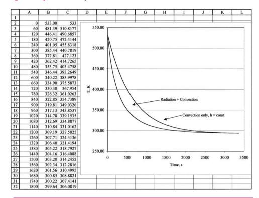
**Figure Example D-6d** | Comparison of results.
