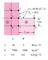
**4-88** Write the transient nodal temperature equation for node 1 in Figure P4-88. Also determine the maximum allowable time increment for the node. The right face is exposed to the convection condition shown. Properties for materials A and B are given in the figure.
