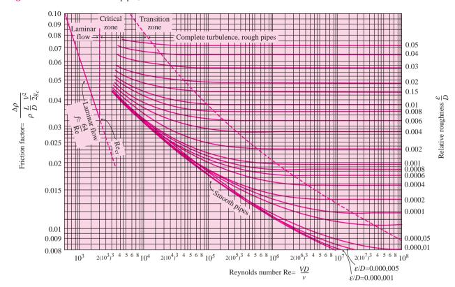
**Figure 6-4** | Friction factors for pipes, from Reference 5.
