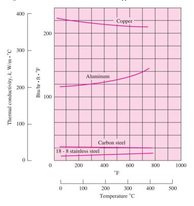
**Figure 1-6** | Thermal conductivities of some typical solids.
