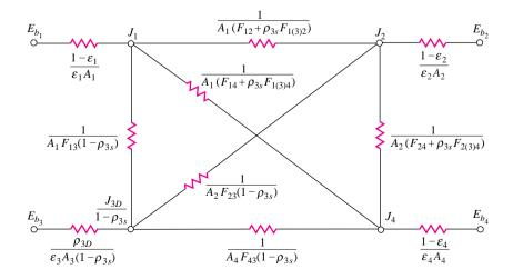
Figure 8-51 | System with two specular-diffuse surfaces.
