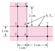
**4-82** Write a steady-state nodal equation for node 3 in Figure P4-82 assuming unit depth perpendicular to the page and using the node spacing shown. The thermal conductivity of the solid is 15 W/m·°C and the convection heat-transfer coefficient on the side surface is 25 W/m<sup>2</sup>·°C.
