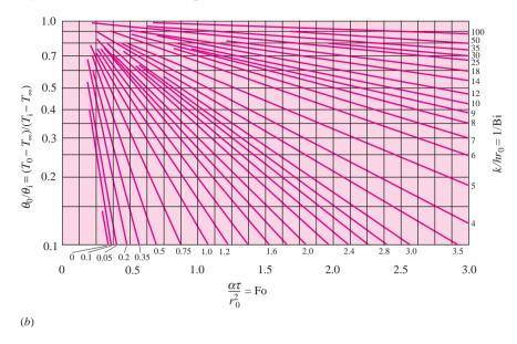
**Figure 4-10** | Temperature as a function of center temperature in an infinite plate of thickness 2*L*, from Reference 2.
