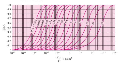
Figure 4-15 | Dimensionlesss heat loss  $Q/Q_0$  of an infinite cylinder of radius  $r_0$  with time, from Reference 6.
