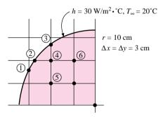
**4-124** Taking Figure P4-124 as a special case of Table 3-2(f), write an explicit formulation for nodes (m, n) and 2 using the resistance-capacity formulation and the information of Table 3-4.
