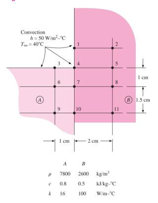
**4-85** For the section shown in Figure P4-85, calculate the maximum time increment allowed for node 2 in a transient numerical analysis. Also write the entire nodal equation for this node.
