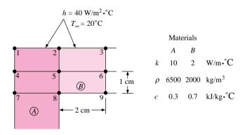
> **4-86** A transient numerical analysis is to be performed on the composite material section shown in Figure P4-86. Calculate the maximum time increment that can be used for node 5 to ensure convergence.
