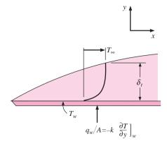
Figure 5-8 | Control volume for integral energy analysis of laminar boundary flow.
