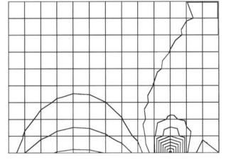
obvious peak at the node containing the heat source, is constant along lower boundaries, and drops off near the convection surface. Plan views of the temperature distribution are also shown in Figure Example D-4(d). The jagged behavior of some of the isotherms results from the relatively coarse grid and the interpolation scheme of the software. Use of a finer grid structure would produce smoother curves.
