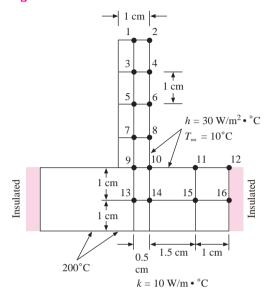
**3-58** Calculate the steady-state temperatures for nodes 1 to 9 in Figure P3-58.
