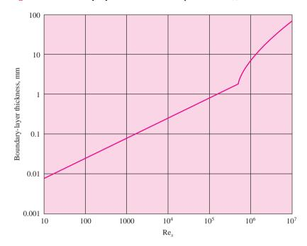
**Figure 5-14** | Boundary-layer thickness for atmospheric air at  $u_{\infty} = 30$  m/s.
