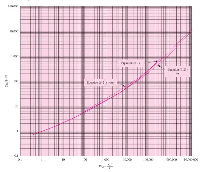
Figure 12-7 | Nusselt numbers for cross flow over isothermal spheres. Properties evaluated at free-stream temperature  $T_{\infty}$ , except  $\mu_w$ .
