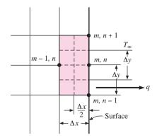
Figure 3-8 | Nomenclature for nodal equation with convection at a corner section.
