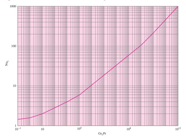
**Figure 7-5** | Free-convection heat transfer from vertical isothermal plates.
