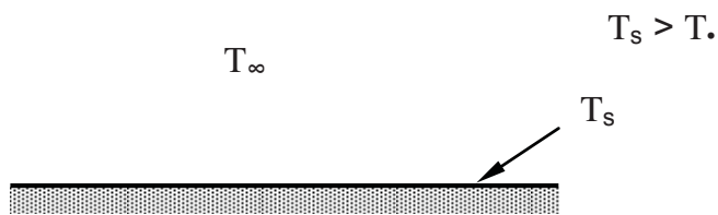
Figure 3-12 Natural convection over a horizontal flat plate
