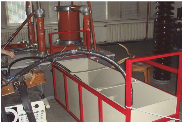
Fig. 15. Experimental set-up for 0.6/1 kV cable.
