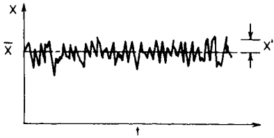
FIGURE 1.7 Property variation with time at some point in a turbulent boundary layer.
