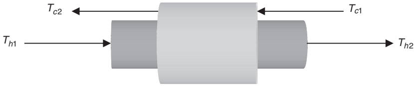
Figure 3.8 Section of a double-pipe exchanger.
