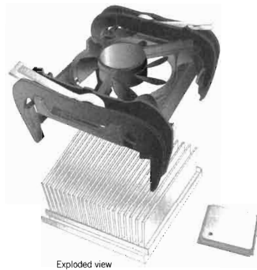
FIGURE 1.11 A finned heat sink and fan assembly (left) and microprocessor (right).
