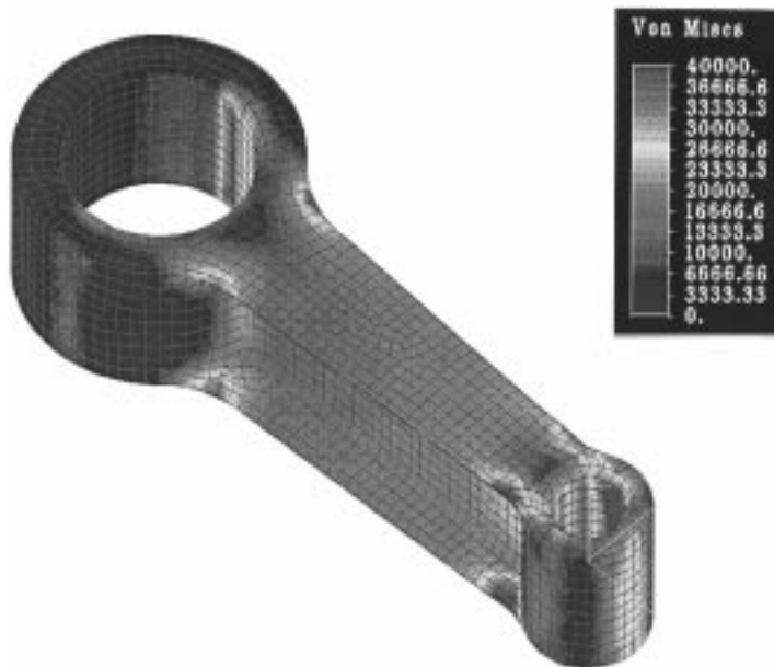
FIGURE 15.5.8 Stress contours and geometry of optimized rod.
