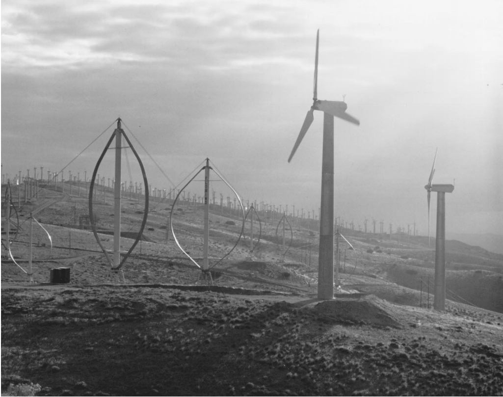
FIGURE 8.11.2 Wind farm both horizontal-axis and vertical-axis turbines.
