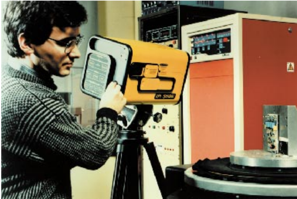
PLATE 3 Vibration screening of a circuit board using an electromagnetic shaker and a laser doppler vibration pattern imager. (Photo courtesy Ometron Inc., Sterling, VA.)
