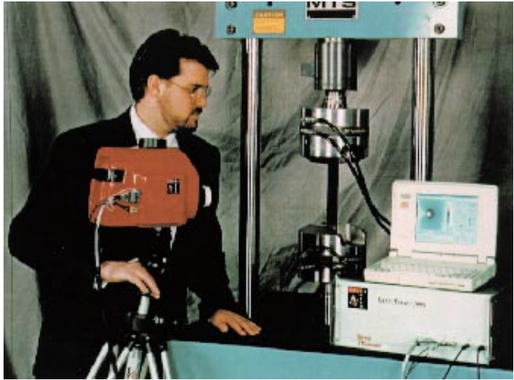
PLATE 11 Delta Therm 1000 Stress Imaging System with principal inventor Jon R. Lesniak. R&D 100 Award-winning instrument in 1994. (Photo courtesy Stress Photonics Inc., Madison, WI.)
