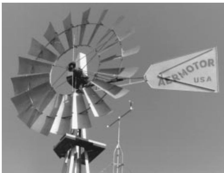
FIGURE 7.7.1 The multiblade American windmill Photograph by Paul Gipe. (Adapted from Wind Power for Home & Business , Chelsea Green Publishing, 1993).
