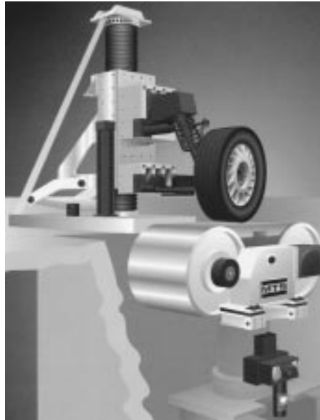
FIGURE 1.1.1 Artist's concept of a moving stainless steel roadway to drive the suspension system through a spinning, articulated wheel, simulating three-dimensional motions and forces. (MTS Systems Corp., Minneapolis, MN. With permission.) Notes: Flat-Trac® Roadway Simulator, R&D100 Award-winning system in 1993. See also Color Plate 1.*
