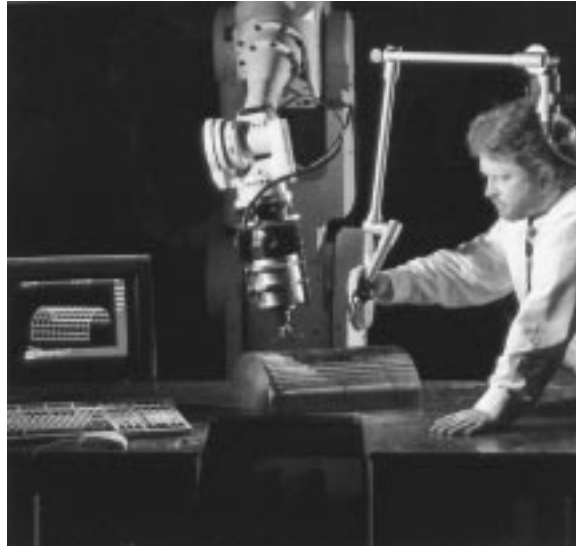
FIGURE 14.11.6 Workpiece surface is digitized and modeled in preparation for automatic tool path generation. (Courtesy of The Automation and Robotics Research Institute, The University of Texas at Arlington.)
