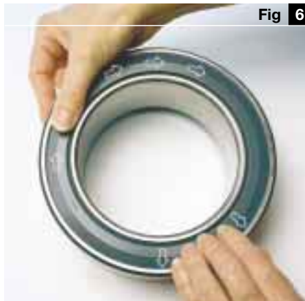
Inserting the seal in the outer ring
