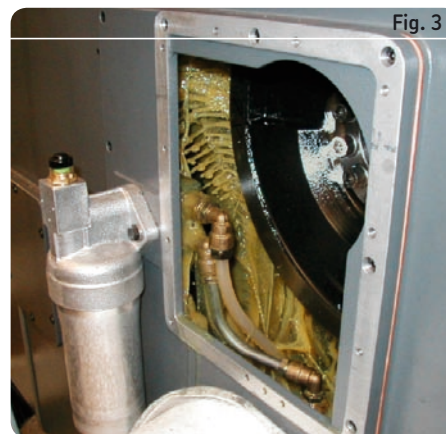
Circulating oil system
