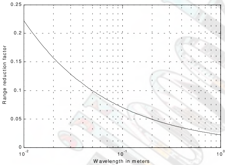
Figure 1.27. Range reduction factor versus radar operating wavelength. This plot was generated using the function “ range_red_factor.m ”.
