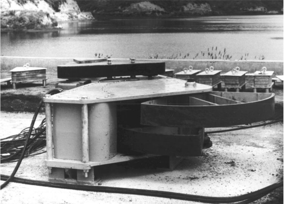
Figure 3.3.1 Counterrotating eccentric weight vibration generator.
