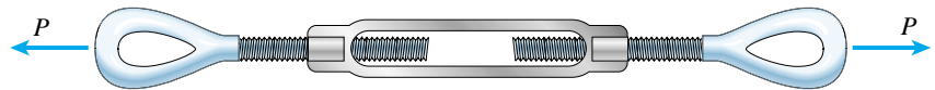
FIG. 2-28 Double-acting turnbuckle. (Each full turn of the turnbuckle shortens or lengthens the cable by 2p , where p is the pitch of the screw threads.)
