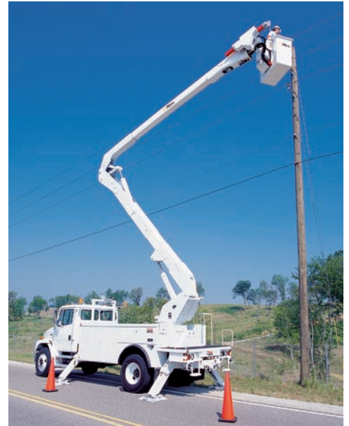
Photo 10.1 The forces exerted by the hydraulic cylinders to position the bucket lift shown can be effectively determined using the method of virtual work since a simple relation exists among the displacements of the points of application of the forces acting on the members of the lift.
