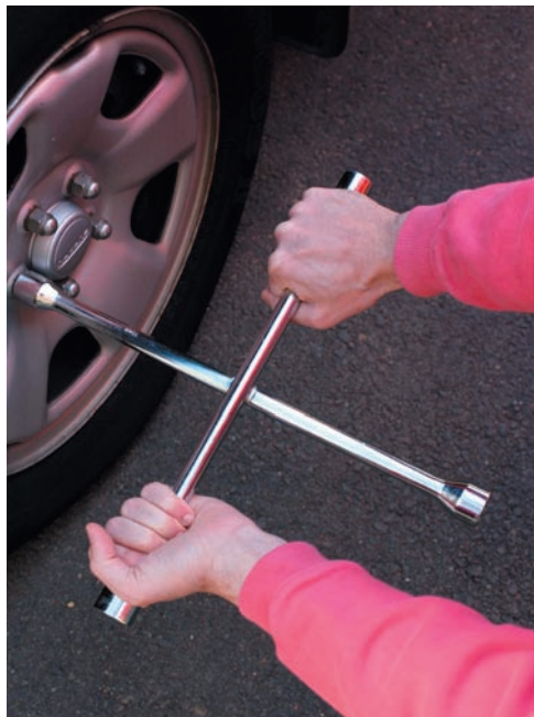
Photo 3.1 The parallel upward and downward forces of equal magnitude exerted on the arms of the lug nut wrench are an example of a couple.
