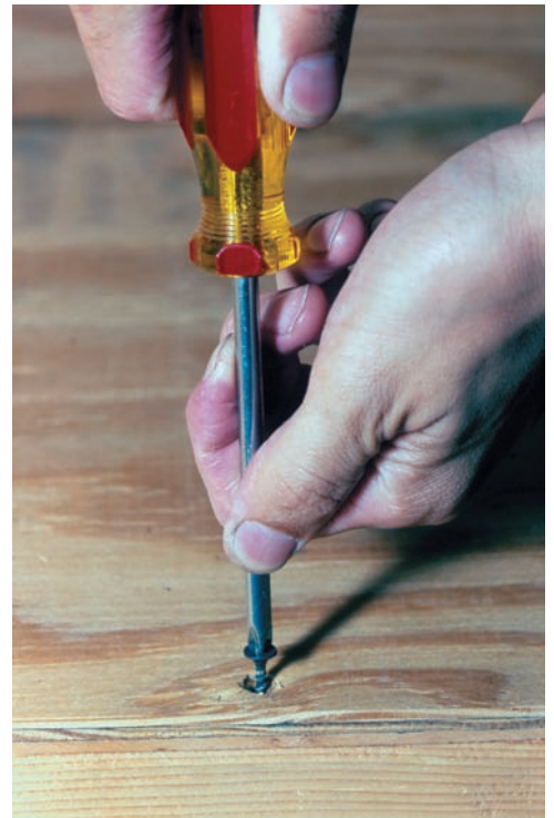
Photo 3.5 The pushing-turning action associated with the tightening of a screw illustrates the collinear lines of action of the force and couple vector that constitute a wrench.
