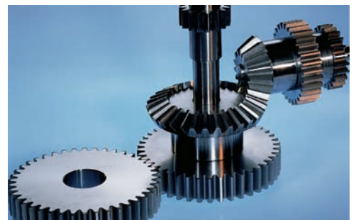
Photo 15.2 For the central gear rotating about a fixed axis, the angular velocity and angular acceleration of that gear are vectors directed along the vertical axis of rotation.
