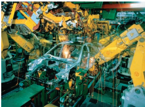
Photo 18.1 The design of a robotic welder for an automobile assembly line requires a three-dimensional study of both kinematics and kinetics.
