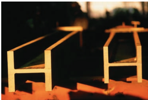
Photo 9.1 Figure 9.13 tabulates data for a small sample of the rolled-steel shapes that are readily available. Shown above are two examples of wide-flange shapes that are commonly used in the construction of buildings.
