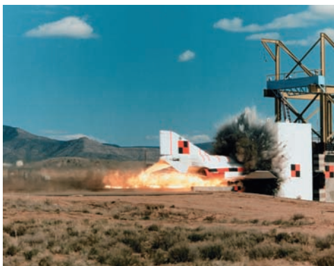
Photo 13.2 This impact test between an F-4 Phantom and a rigid reinforced target was to determine the impact force as a function of time.
