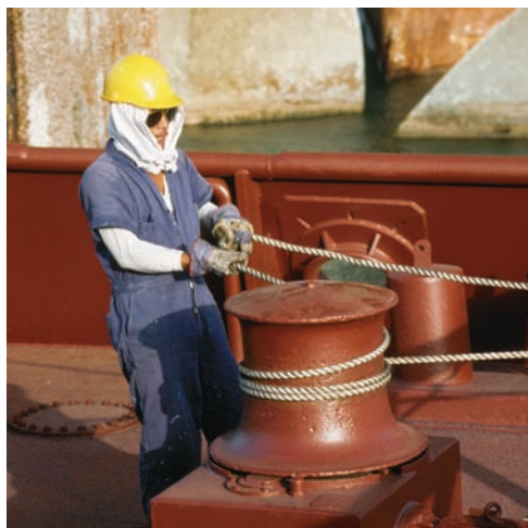
Photo 8.3 By wrapping the rope around the bollard, the force exerted by the worker to control the rope is much smaller than the tension in the taut portion of the rope.
