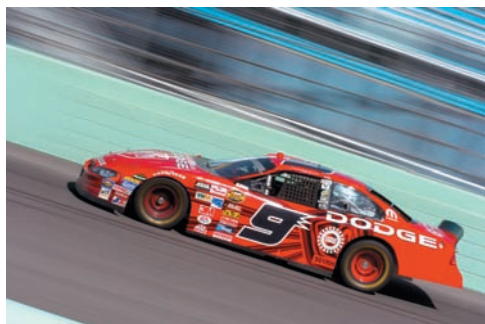
Photo 15.5 If the tires of this car are rolling without sliding the instantaneous center of rotation of a tire is the point of contact between the road and the tire.
