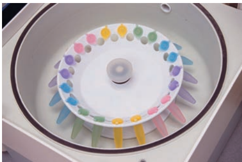
Photo 12.4 The forces on the specimens used in a high speed centrifuge can be described in terms of radial and transverse components.
