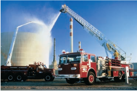
Photo 15.8 When the ladder rotates about its fixed base, its angular velocity can be obtained by adding the angular velocities which correspond to simultaneous rotations about two different axes.
