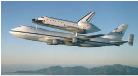
Photo 5.4 To predict the flight characteristics of the modified Boeing 747 when used to transport a space shuttle, the center of gravity of each craft had to be determined.
