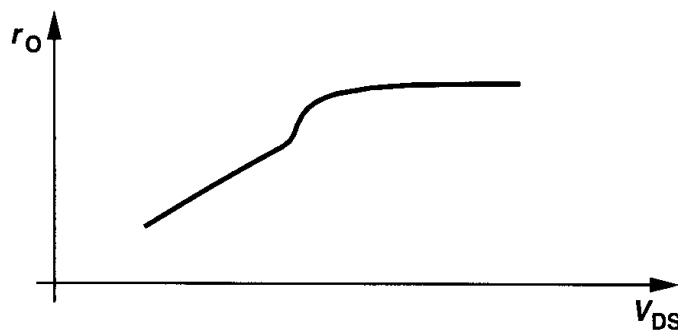
Figure 16.14 Kink in output resistance in Level 3 model.
