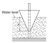
The conical float is free to slide on a vertical rod. When the float is disturbed from its equilibrium position, it undergoes oscillating motion described by the differential equation
