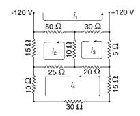
Determine the loop currents  $i_1$  to  $i_4$  in the electrical network shown.
