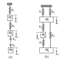
13. ■ The displacement formulation for the mass–spring system shown in Fig. (b) results in the following equilibrium equations of the masses:
