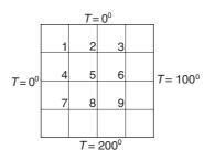
The edges of the square plate are kept at the temperatures shown. Assuming steady-state heat conduction, the differential equation governing the temperature T in the interior is
