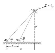
The radar stations *A* and *B*, separated by the distance a = 500 m, track the plane *C* by recording the angles  $\alpha$  and  $\beta$  at one-second intervals. If three successive readings are
