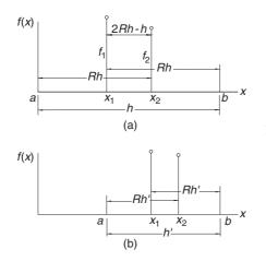
Figure 10.2. Golden section telescoping.
