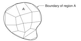
**Figure 6.6.** Finite element model of an irregular region.
