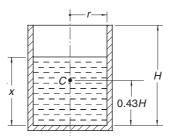
The cylindrical vessel of mass *M* has its center of gravity at *C*. The water in the vessel has a depth *x*. Determine *x* so that the center of gravity of the vessel–water combination is as low as possible. Use M = 115 kg, H = 0.8 m and r = 0.25 m.
