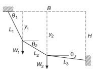
A cable supported at the ends carries the weights  $W_1$  and  $W_2$ . The potential energy of the system is
