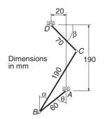
Geometric analysis of the linkage shown resulted in the following table relating the angles  $\theta$  and  $\beta$ :
