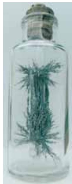
Fig. 28-4 (a) The magnetic field lines for a bar magnet. (b) A “cow magnet”—a bar magnet that is intended to be slipped down into the rumen of a cow to prevent accidentally ingested bits of scrap iron from reaching the cow’s intestines. The iron filings at its ends reveal the magnetic field lines. (Courtesy Dr. Richard Cannon, Southeast Missouri State University, Cape Girardeau)
