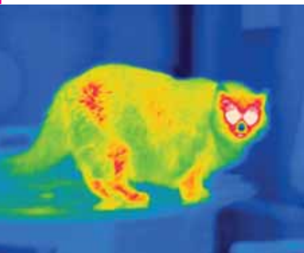
Fig. 18-20 A false-color thermogram reveals the rate at which energy is radiated by a cat. The rate is color-coded, with white and red indicating the greatest radiation rate. The nose is cool. (Edward Kinsman/Photo Researchers)
