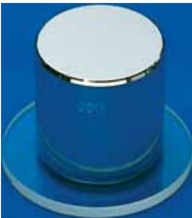
Fig. 1-3 The international 1 kg standard of mass, a platinum–iridium cylinder 3.9 cm in height and in diameter. (Courtesy Bureau International des Poids et Mesures, France)
