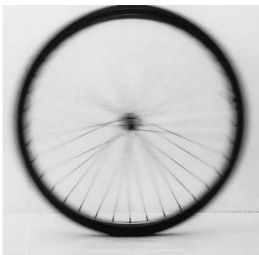
Fig. 11-5 A photograph of a rolling bicycle wheel. The spokes near the wheel's top are more blurred than those near the bottom because the top ones are moving faster, as Fig. 11-4c shows. (Courtesy Alice Halliday)
