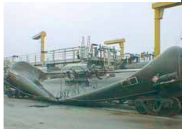
Fig. 19-1 A railroad tank car crushed overnight. (Photo courtesy www.Houston.RailFan.net )
