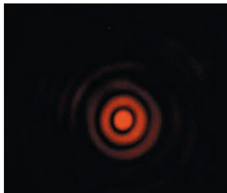
Fig. 36-3 A photograph of the diffraction pattern of a disk. Note the concentric diffraction rings and the Fresnel bright spot at the center of the pattern. This experiment is essentially identical to that arranged by the committee testing Fresnel's theories, because both the sphere they used and the disk used here have a cross section with a circular edge. (Jearl Walker)
