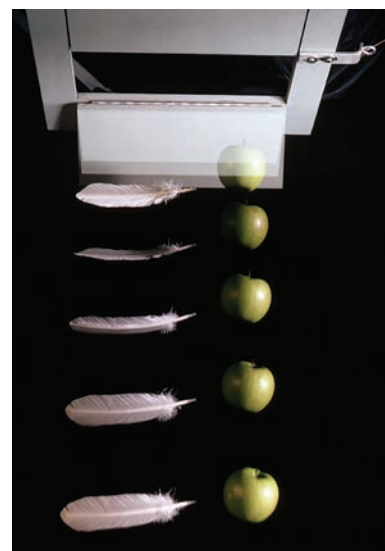
Fig. 2-10 A feather and an apple free fall in vacuum at the same magnitude of acceleration g . The acceleration increases the distance between successive images. In the absence of air, the feather and apple fall together. (Jim Sugar/Corbis Images)
