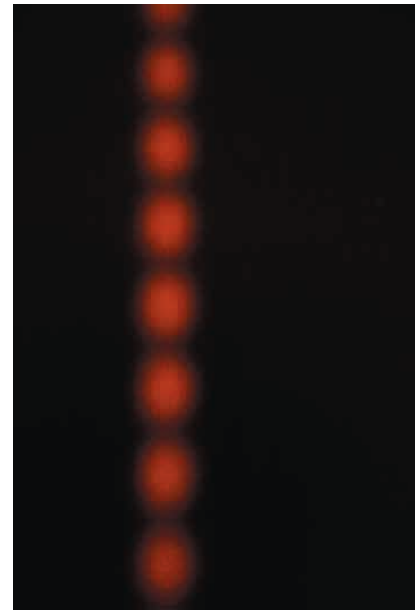
Fig. 35-9 A photograph of the interference pattern produced by the arrangement shown in Fig. 35-8, but with short slits. (The photograph is a front view of part of screen C .) The alternating maxima and minima are called interference fringes (because they resemble the decorative fringe sometimes used on clothing and rugs). (Jearyl Walker)
