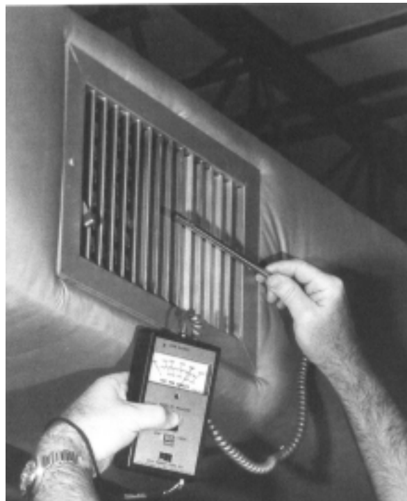
Figure 3-5. Proper use of an air velocity meter (Courtesy, Dwyer Instruments, Inc.)
