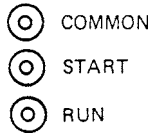
Fig. 7-45 Built-up terminals on pancake compressors manufactured before 1952. (Tecumseh)
