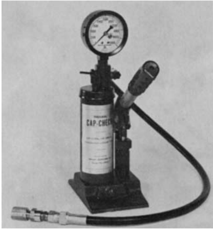
Fig. 1-50 Cap-Check is a portable self-contained hydraulic power unit with auxiliary equipment that is especially adapted to cleaning refrigeration capillary tubes. It is hand operated.
