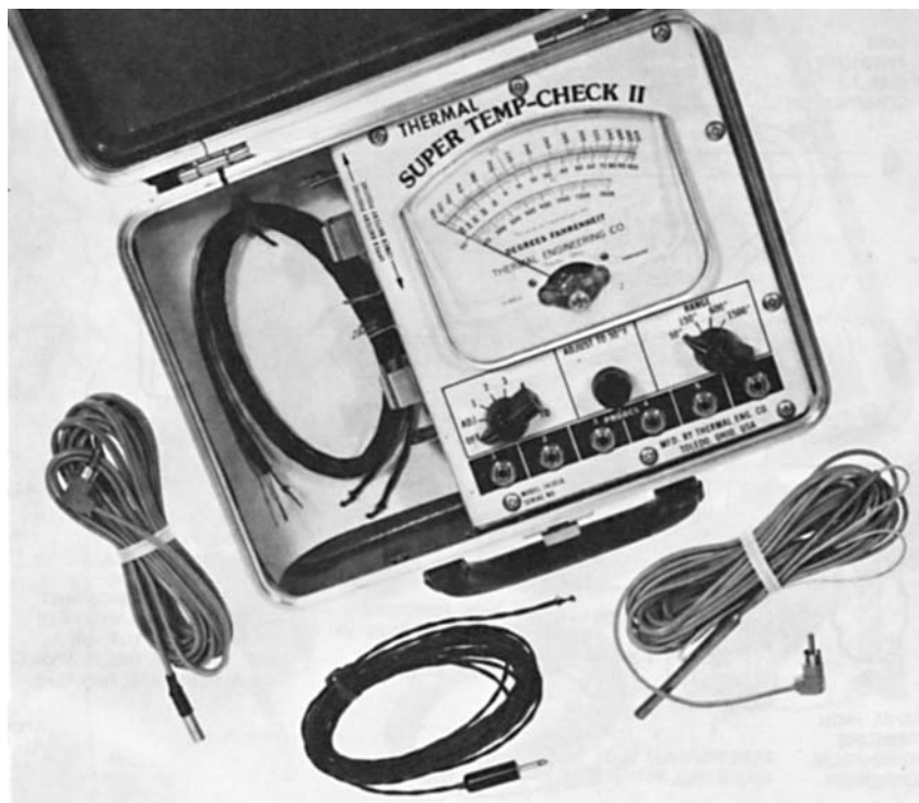
Fig. 1-33 Electronic thermometer for measuring superheat. The probes are made of thermo-couple wire. They can be strapped on anywhere with total contact with the surface. This thermometer covers temperatures from -50^{\circ} to 1500^{\circ}\text{F} on four scales. The temperature difference between any two points directly means it can read superheat directly. It is battery operated and has a \pm 2 percent accuracy on all ranges. Celsius scales are available. (Thermal Engineering)
