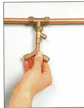
Draincock key A special tool, similar in principle to a radiator-valve key, is available for operating draincocks.
