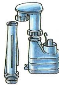
Three-part siphon ▶ This type of siphon can be dismantled for replacement of the flap valve without having to shut off the water or drain the cistern.
