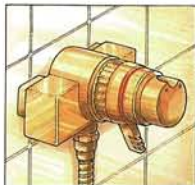
Thermostatic mixer This unit prevents excessive fluctuations in water temperature.
