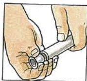
2 Insert metal sleeve
