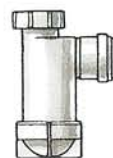
Bottle trap This type of trap can be cleared easily because the whole base of the trap unscrews by hand.
