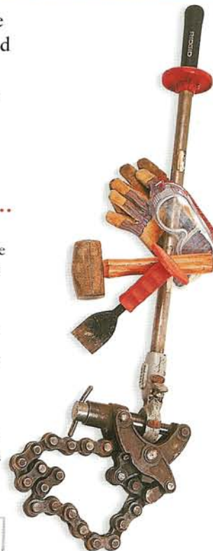
Cutting a soil pipe Use a chain-link cutter to cut a broken soil pipe square.
