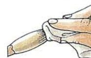
Smoothing epoxy putty When patching a hole with epoxy putty, smooth it with a damp soapy cloth to give a neat finish.
