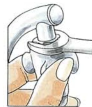
1 Loosen locking nut
