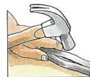
Closing a split pipe In an emergency, close a split by tapping the pipe with a hammer before you bind it. This works particularly well with lead pipe.
