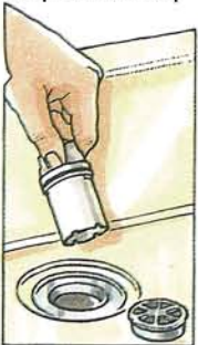
Cleaning compact traps Compact traps for showers have a lift-out dip tube for easy cleaning.
