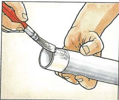
5 Paint solvent up to the pencil mark
