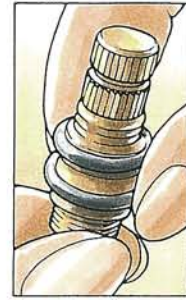
2 Roll ring from groove
