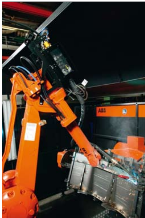
Figure 3. Overview of mud screen assembled with many short welds.
