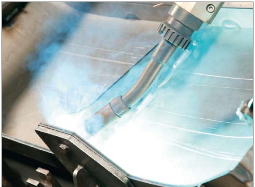
Figure 2. Mud screen assembled with short intermittent welds with good cosmetic appearance.
