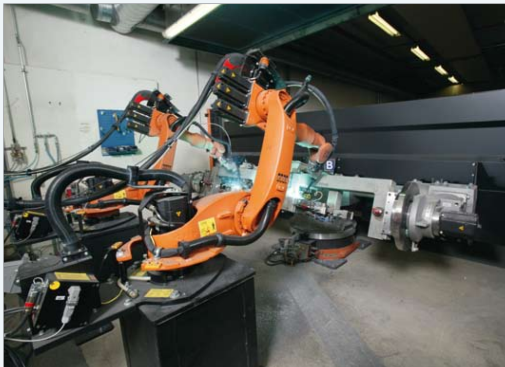
Figure 1. Welding station for cross beams.
