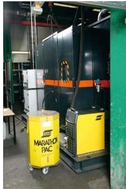
Figure 4. Aristo Mig 5000i inverter and 275kg Marathon Pac installed outside the Flexarc robot cell.
