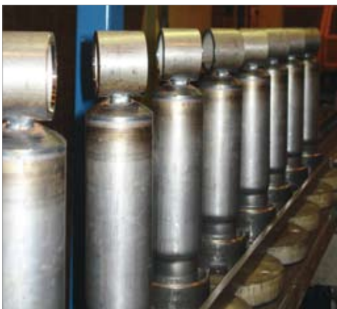
Figure 2. Shock absorber housings with welded assembly ring.
