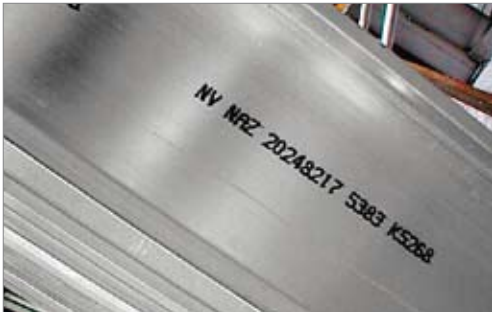
Figure 9. The 5383 base material with higher strength to weight than 5083 material, is welded with 5183 type welding wire from AlcoTec.
