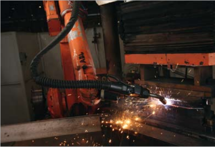
Figure 3. Cell for the robotic welding of catalytic converters.
