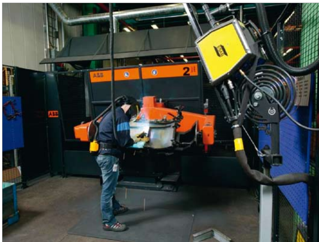
Figure 5. Manual tack welding. Aristo Mig 4000i power source located outside the Flexarc cell.
