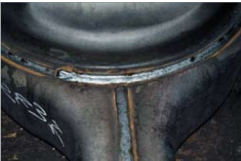
Figure 6. After welding, the axle housing is clean.
