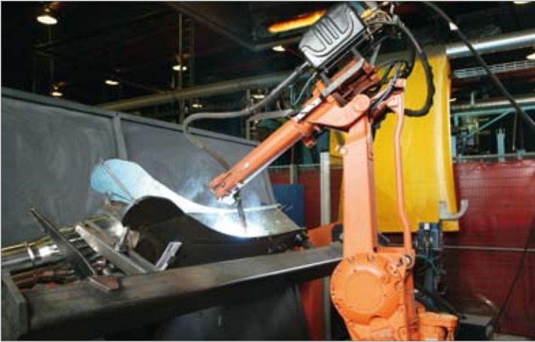
Figure 3. OK Tubrod 14.11-1.2mm applied for welding loader bodies with limitations to the amount of weld metal deposited. A mix of small fillet welds and circular welds.
