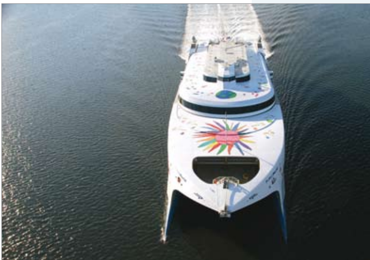
Figure 1. Natchan World's highly efficient wave piercing bows produce very low wake.
