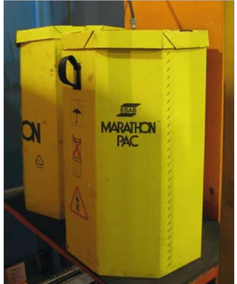
Figure 2. Two octagonal Marathon Pacs with OK AristoRod 12.50 (AWS class ER70S-6) copper-free wire installed behind a robotised welding cell 25 feet away from the contact tip without feeding issues.
