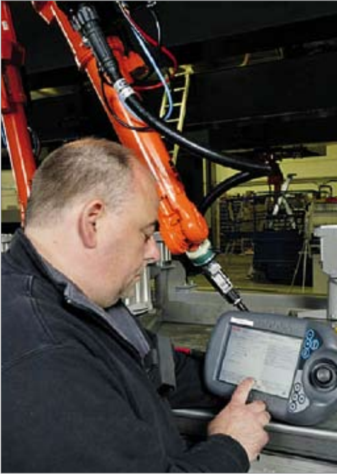
Figure 3. All programming, both for the robot and the welding equipment, is done with the IRC5 control unit.
