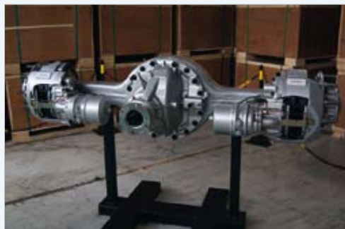
Figure 1. Typical heavy truck rear axle, with disc brakes.
