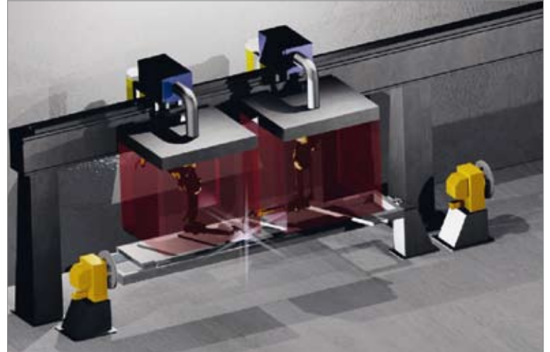
Figure 2. One side of a gantry welding station during test welding at Andon. The complete station consists of two welding tables with fixtures, one gantry, two suspended IRB2400L ABB robots equipped with the ESAB W8 Robot package, including two Marathon Pac bulk drums with 250 kg of OK Autrod 12.51 MAG wire.
