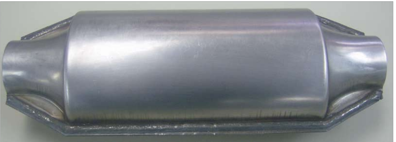
Figure 5. Converter welded with Arcaloy 409Ti.
