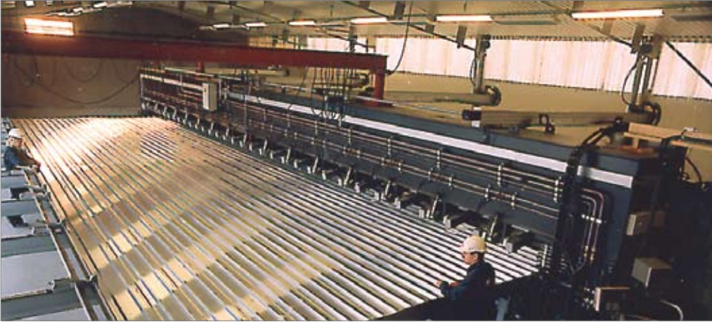
Figure 2. The world's first industrial FSW machine; installed at Marine Aluminium in 1996 and, since then, producing panels for marine applications.
