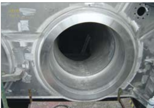
Figure 13. To manage propulsion nozzle flange distortion welding operations are performed before milling.
