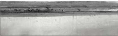
Figure 3. Overlap joint in 1.2mm zinc coated plate (layer thickness < 10\mu\text{m} ). Shielding gas: M20 (92%Ar / 8% \text{CO}_2 ); 240A, 21V; V_s=170\text{cm/min} .
