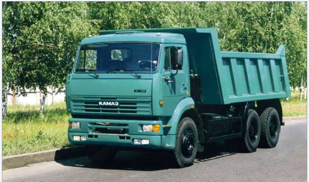
Figure 1. The KAMAZ 6520 dumpster truck. Note the lateral wall with reinforcements for which the robotic welding stations have been designed.
