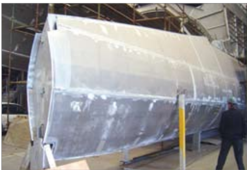
Figure 12. Rigid wave piercing bows have some skin sections up to 25mm.
