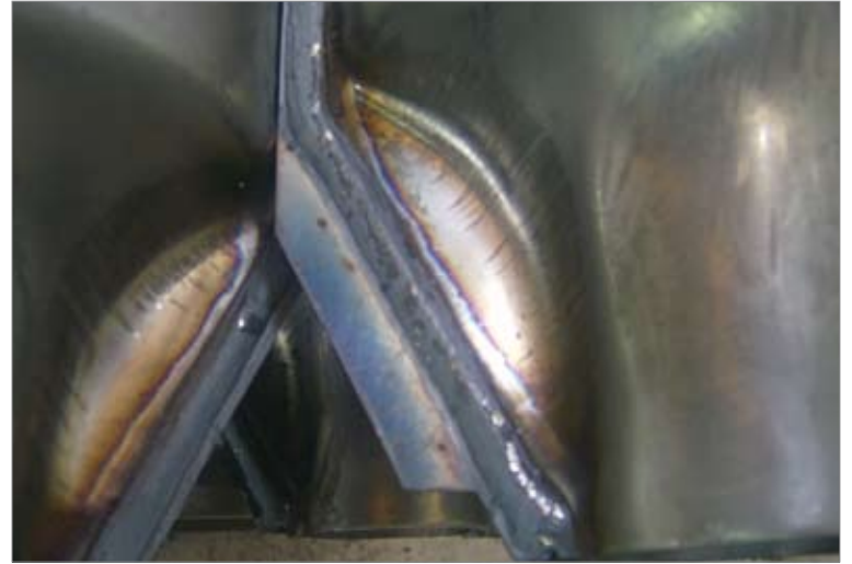
Figure 4. Detail of converter welded with Arcaloy 409Ti.
