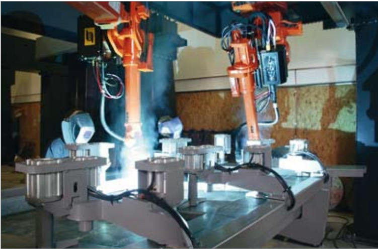
Figure 2. One side of a gantry welding station during test welding at Andon. The complete station consists of two welding tables with fixtures, one gantry, two suspended IRB2400L ABB robots equipped with the ESAB W8 Robot package, including two Marathon Pac bulk drums with 250 kg of OK Autrod 12.51 MAG wire.
