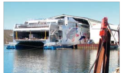
Figure 15. Incat's final assembly building hull troughs are flooded for hull 65 to slip the shed.
