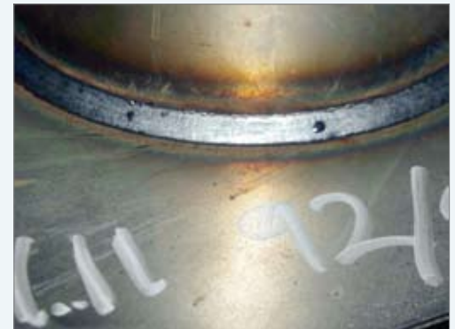
Figure 1. Circular fillet weld. t=2 mm, 280A, 22V, 150cm/min.
