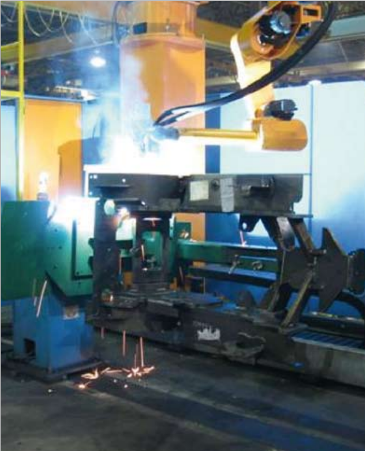
Figure 1. Forklift frame welded with GMAW-P process, using OK AristoRod 12.50 copper-free wire, diameter 1.2 mm in 90% Ar/10% CO 2 shielding gas. The low spatter level helps to keep the weldment, fixtures and welding equipment clean.
