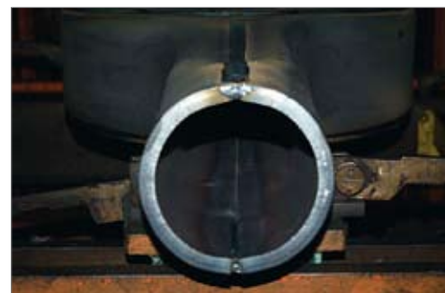
Figure 5. Full penetration by one-sided welding.
