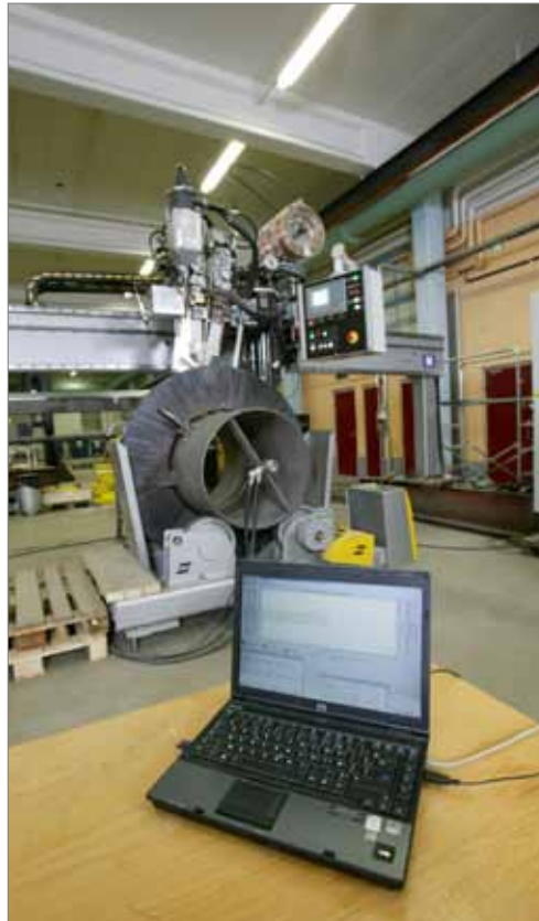
Loading and positioning can be done easily with ESAB's self-aligning or manually adjusted roller beds.
