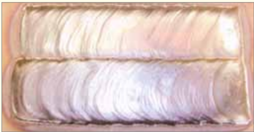
Full weld bead cladded with OK Flux 10.31/OK Band 7018). ESAB A6 head, 2 x ESAB LAF 1600 DC, PEH control unit. 1000A / 30V / 13 cm/min, DC+. All welds are free of surface defects.
