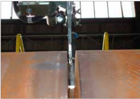
Figure 7. A view into the gap of the assembled joint before the start of the process.
