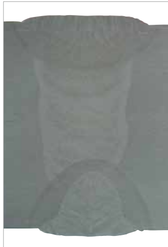
Figure 4 (left). Macro of narrow gap welding seam for GMAW (production test weld for the Nord Stream project). The opening angle is 3 degrees from the root and zero degrees from the centre.
