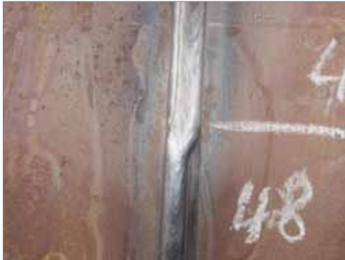
Figure 11. Automatic overlapping and bead shift after each revolution.
