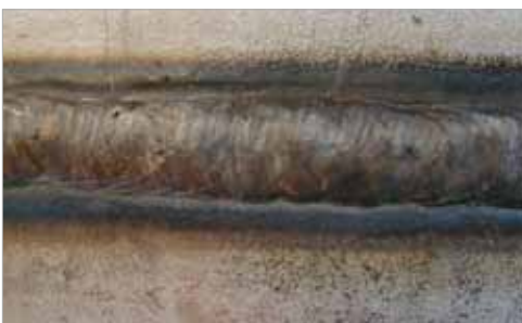
Figure 5. One run PC joint with OK Autrod 308LSi.
