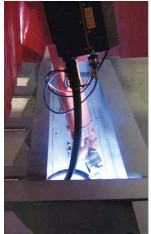
Figure 3. Close corner welding made possible by smart sensors and programming software.
