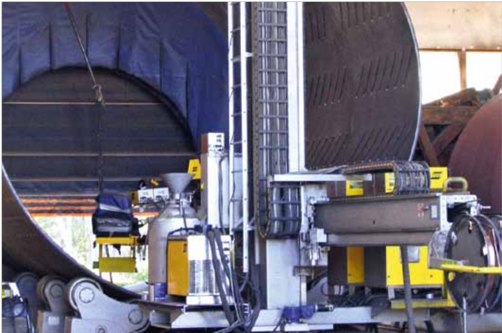
Figure 3. SAW column and boom is fitted for tandem welding, used extensively in the welding of peeling drums and other heavy-duty products.
