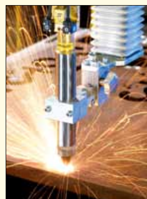
Patented torch with automatic internal ignition, recommended for all automated production processes.
