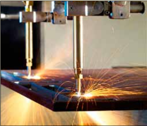
Innovative construction of the JETCON™ nozzle holder, allows it to be changed in an instant. The inherent long lifetime of the nozzle holder greatly reduces wear part consumption.
