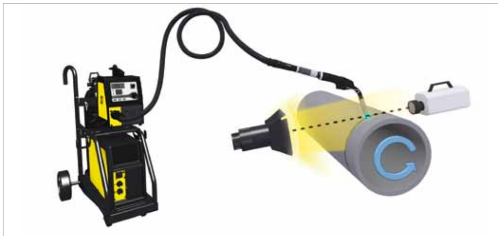
Figure 6. Set-up used for high current welding tests
