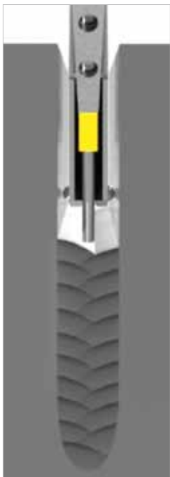
Figure 3: Standard narrow gap joint weld beads graphics.
