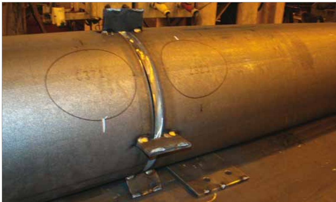
Figure 3. Pipe ends prepared for butt welding. Note the graphics instructions for joining pipes (number, location and orientation).
