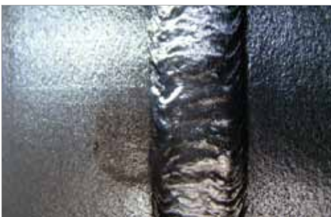
Figure 6. Shield-Bright 308L cover-layer after pickling.
