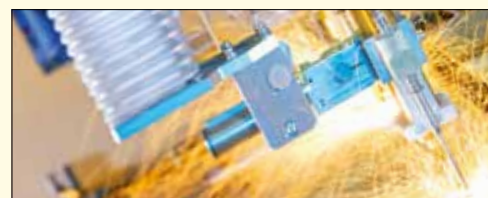
Patented torch with automatic internal ignition, recommended for all automated production processes.
