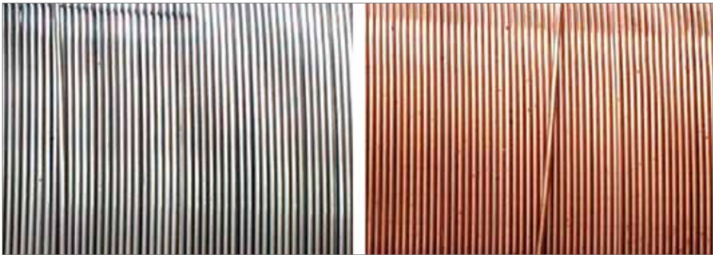
Figure 11. Wire surface after 6 days of unprotected exposure at 80% relative humidity and 26.6°C. Left OK AristoRod™, right copper coated wire. Source: ISF Aachen.
