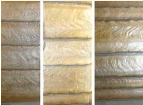
Cladding with OK Band NiCu7 strip on mild steel plate. DC+, 800A, 29V, 13cm/min.
