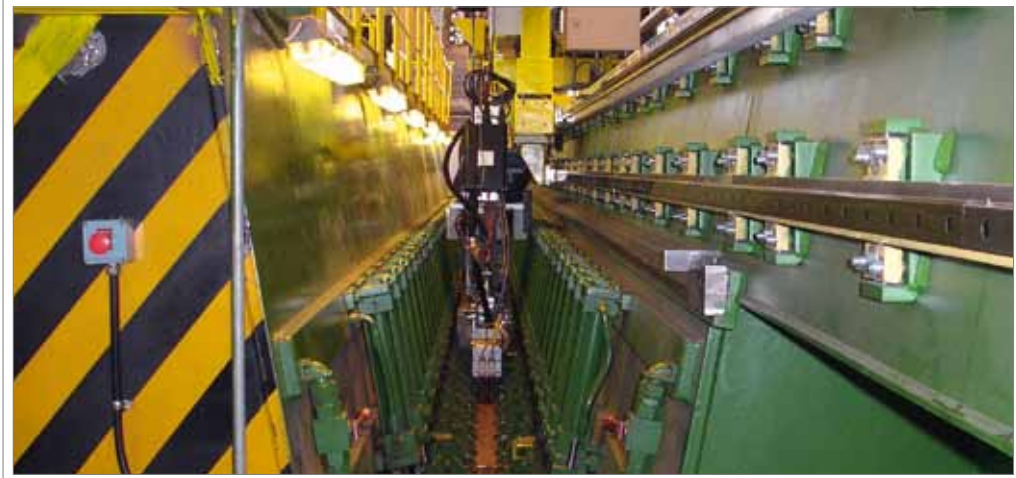
Laser hybrid welding station and a complete hybrid weld.
