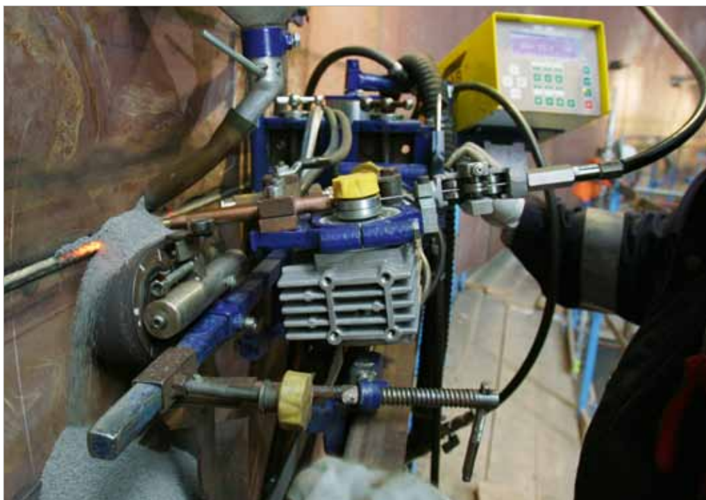
Figure 11. Close-up of the SAW welding in PC position. A rotating belt keeps the weld pool protected by flux. The same procedure is first executed on the outside of the tank, after which the root area is ground to prepare for the inside weld.
