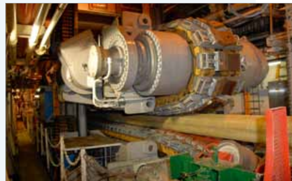
Figure 1. One of three 350 t tensioners onboard Allseas' Solitaire lay barge.
