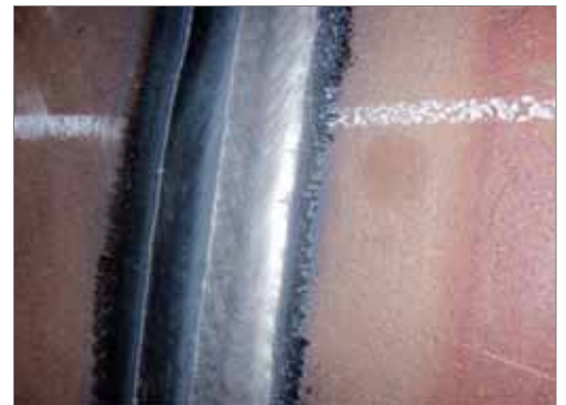
Figure 12. Cap layers of the narrow gap joint.
