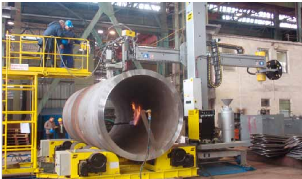
Figure 6. Overview of the submerged arc welding station for circumferential welds.
