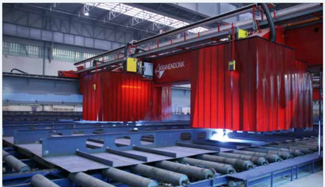
Figure 1. Four robots welding simultaneously with no possibility of collision. Two gantries over a 35 x 16.5 m wide panel.
