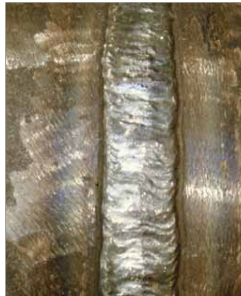
Figure 6. Joint welded with OK Tubrod 15.14 all-positional rutile cored wire. Note the spatter free area adjacent to the joint and the completely self-released slag.
