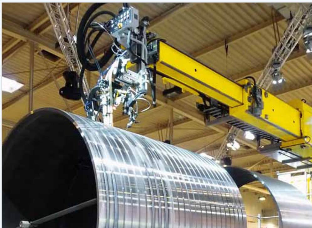
The space saving ESAB telescopic column and boom - Telbo™.
