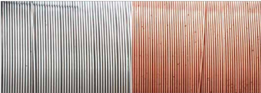
Figure 12. Wire surface after 14 days of unprotected exposure at 80% relative humidity and 26.6°C. Left OK AristoRod™, right copper coated wire. Source: ISF, Aachen.
