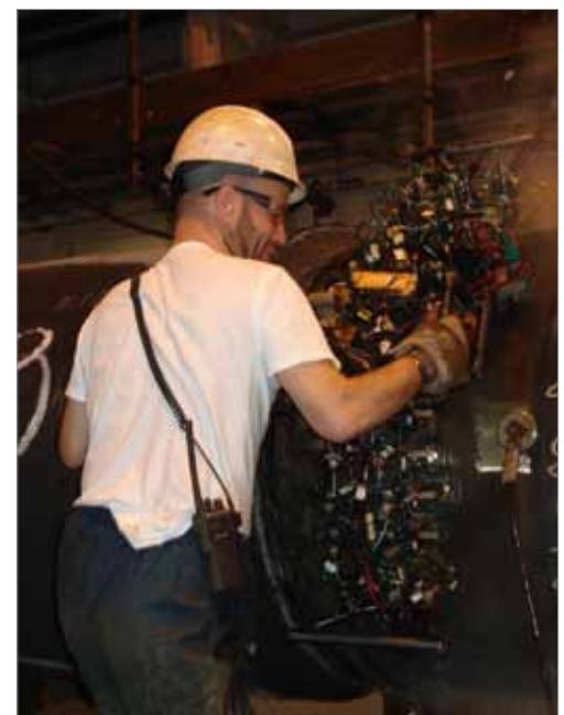
Figure 6. Automatic ultrasonic testing with pulse echo.
