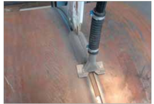
Figure 9. Exhaustion of unconsumed flux from the surface of the joint.
