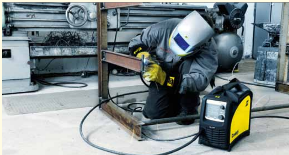
Figure 5: Welding slip-off protection bars to a rack in the workshop.
