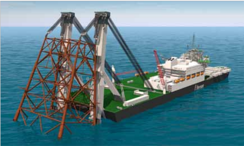
Figure 12. Graphical impression of the Pieter Schelte, a combined vessel for pipe lay and installing and dismantling rigs. It will be the biggest of its kind in the world - and uses dynamic positioning.
