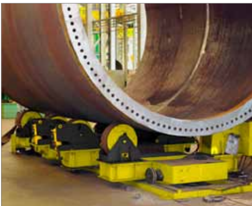
Loading and positioning can be done easily with ESAB's self-aligning or manually adjusted roller beds.
