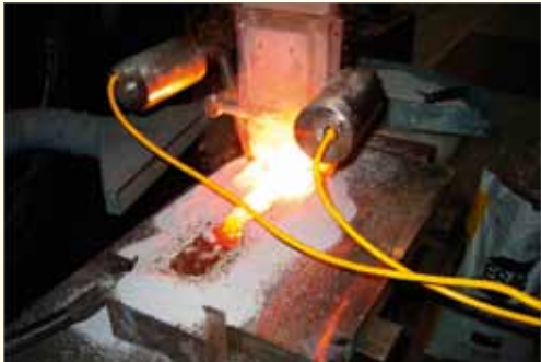
Full weld bead cladded with OK Flux 10.26/OK Band 316L 60 x 0.5mm. All welds free of surface defects. ESAB A6 head, ESAB 2 x LAF 1600 DC, PEH control unit. 1250 A / 24 V/ 18 cm/min; DC+, s/o 35 mm, FH 45 mm.
