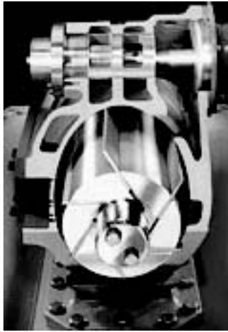
Figure 3.8 Cutaway view of a rotary vane compressor ( Courtesy of Pneumofore SpA ).
