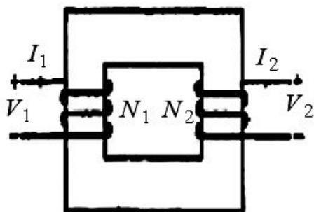
$$V_1 V_2 = N_1 N_2 = I_1 I_2 \quad .2$$
